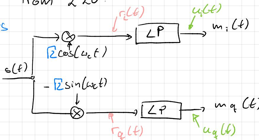
LP with cut-off frequency  $\omega_H < \omega_{c0} < 2\omega_c - \omega_H$
