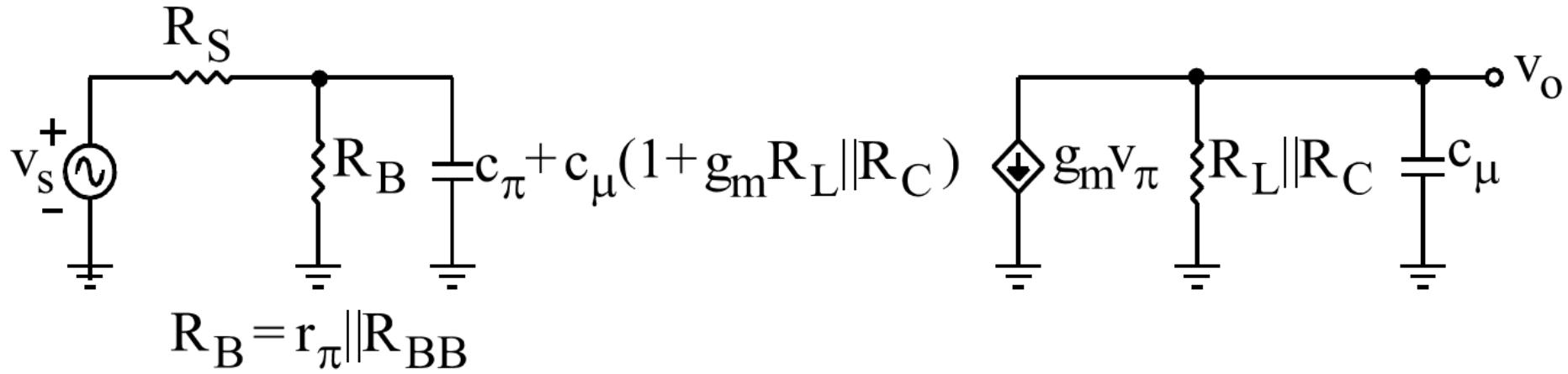
$$F_H(s) = \frac{\frac{1}{R_{BB} || r_\pi || R_S [ c_\pi + c_\mu (1 + g_m R_C || R_L) ]}}{\left( s + \frac{1}{R_{BB} || r_\pi || R_S [ c_\pi + c_\mu (1 + g_m R_C || R_L) ]} \right)} \cdot \frac{\frac{1}{R_C || R_L c_\mu}}{\left( s + \frac{1}{R_C || R_L c_\mu} \right)}$$
