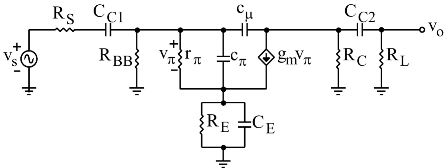
$$F(s) = \underbrace{F_L(s)}_{LF \text{ part}} \underbrace{A_M}_{Midband} \underbrace{F_H(s)}_{HF \text{ part}}$$
