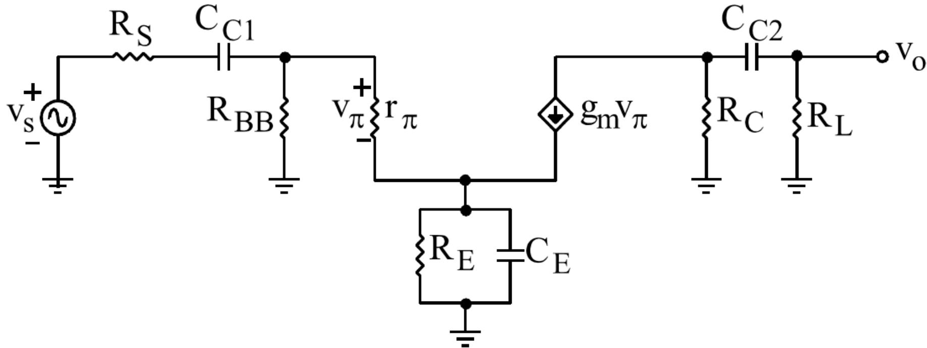
$$F_L(s) \approx \left( \frac{s}{s + \omega_{Lp1}} \right) \left( \frac{s}{s + \omega_{Lp2}} \right) \left( \frac{s + \omega_{Lz3}}{s + \omega_{Lp3}} \right)$$
