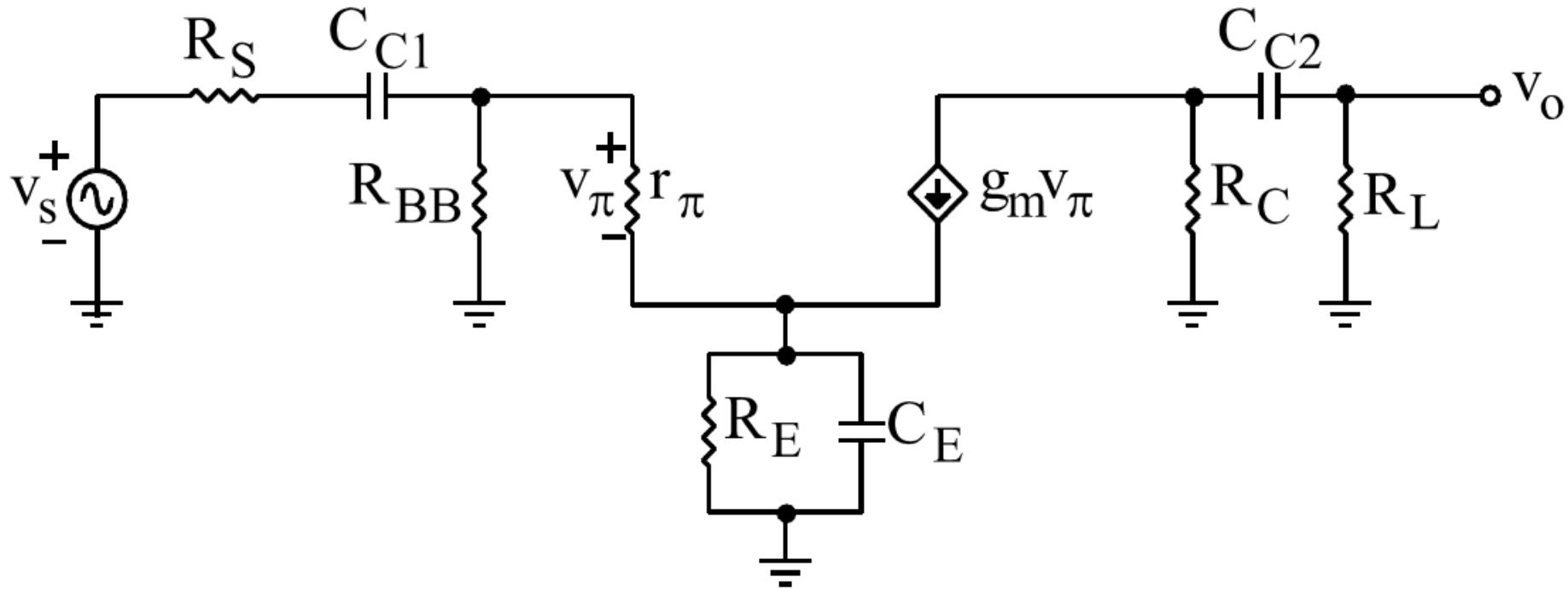
$$\tau_{C_{C2}} = (R_C + R_L) C_{C2} \Rightarrow \omega_{Lp1} = \frac{1}{(R_C + R_L) C_{C2}}$$
