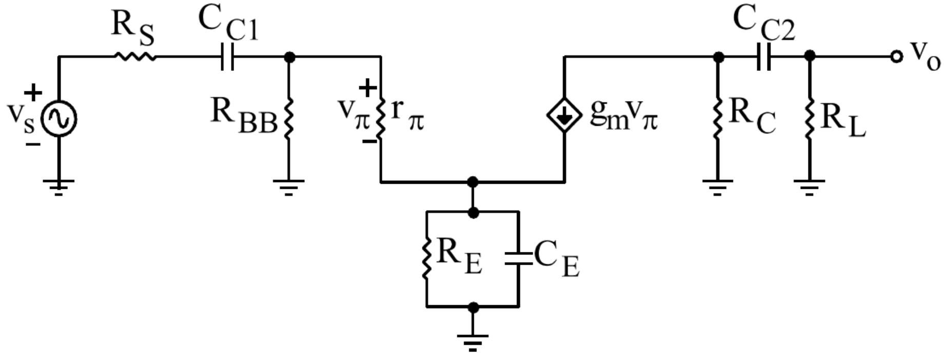
$$\tau_{C_{C1}}^{sc} = (R_S + R_{BB} \parallel r_\pi) C_{C1}$$
