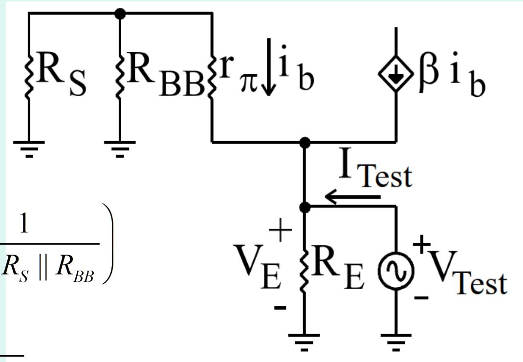
$$\tau_{C_E}^{sc} = \left( R_E \parallel \frac{r_\pi + R_S \parallel R_{BB}}{\beta + 1} \right) C_E$$
