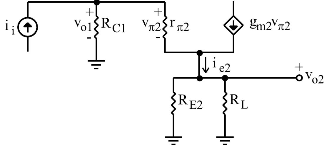
$$R_{o2} = R_{E2} \parallel \frac{r_{\pi 2} + R_{C1}}{\beta_2 + 1} \approx \frac{r_{\pi 2} + R_{C1}}{\beta_2 + 1}$$
