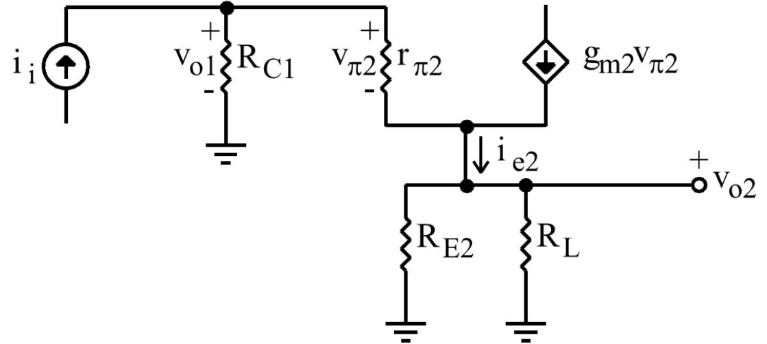
$$v_{o2} = (R_{E2} \parallel R_L) i_{e2} = (R_{E2} \parallel R_L) \frac{(\beta + 1) v_{o1}}{r_{\pi 2} + (\beta + 1) R_{E2} \parallel R_L}$$
