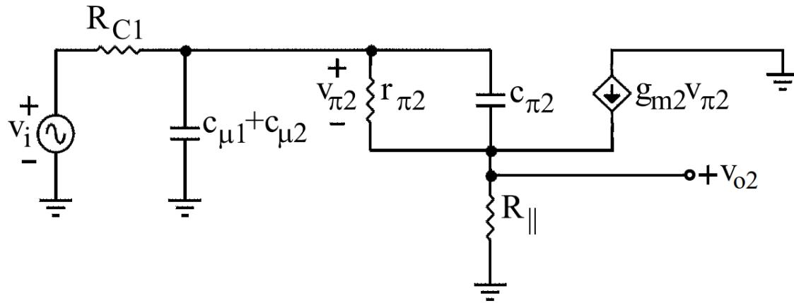
$$v_{o2} = 0 \Leftrightarrow R_{\parallel} (y_{\pi 2} v_{\pi 2} + g_{m2} v_{\pi 2}) = 0 \quad \frac{1}{r_{\pi 2}} + s_{Hz} C_{\pi 2} + \underbrace{\frac{\beta_2}{r_{\pi 2}}}_{g_{m2}} = 0 \Rightarrow s_{Hz} = -\frac{\beta_2 + 1}{r_{\pi 2} C_{\pi 2}}$$
