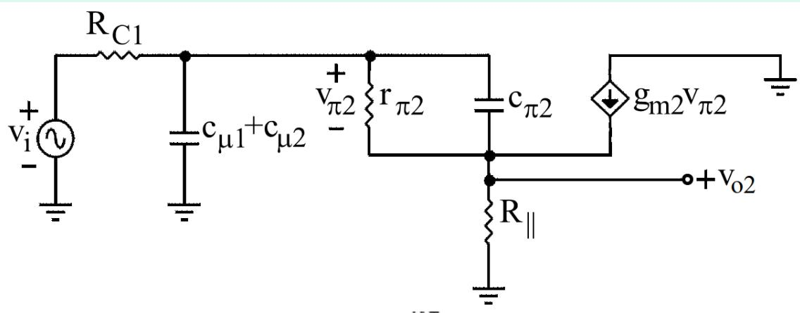
$$\tau_{c\pi 2}^{oc} = \left( c_{\pi 2} \times \frac{r_{\pi 2}}{R_{in2}} \right) \left( R_{C1} \| R_{in2} \right) \left( 1 + \frac{R_{\parallel}}{R_{C1}} \right) \approx$$
