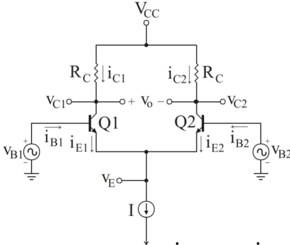
$$v_{B1} = v_{B2} \Rightarrow v_{BE1} = v_{BE2} \Rightarrow \begin{cases} i_{E1} = i_{E2} = \frac{I}{2} \\ i_{C1} = i_{C2} = \alpha \frac{I}{2} \end{cases}$$
