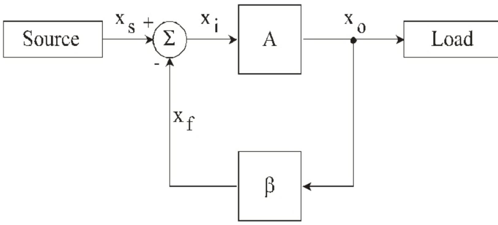
$$\left. \begin{array}{l} x_o = Ax_i \\ x_f = \beta x_o \\ x_i = x_s - x_f \end{array} \right\} \Rightarrow A_f = \frac{x_o}{x_s} = \frac{Ax_i}{x_i + x_f} = \frac{A}{1 + A\beta}$$
