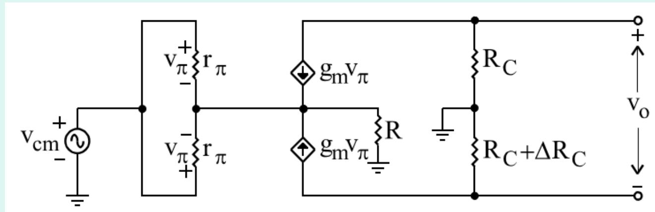
$$v_o = -g_m v_\pi [R_C - (R_C + \Delta R_C)]$$
