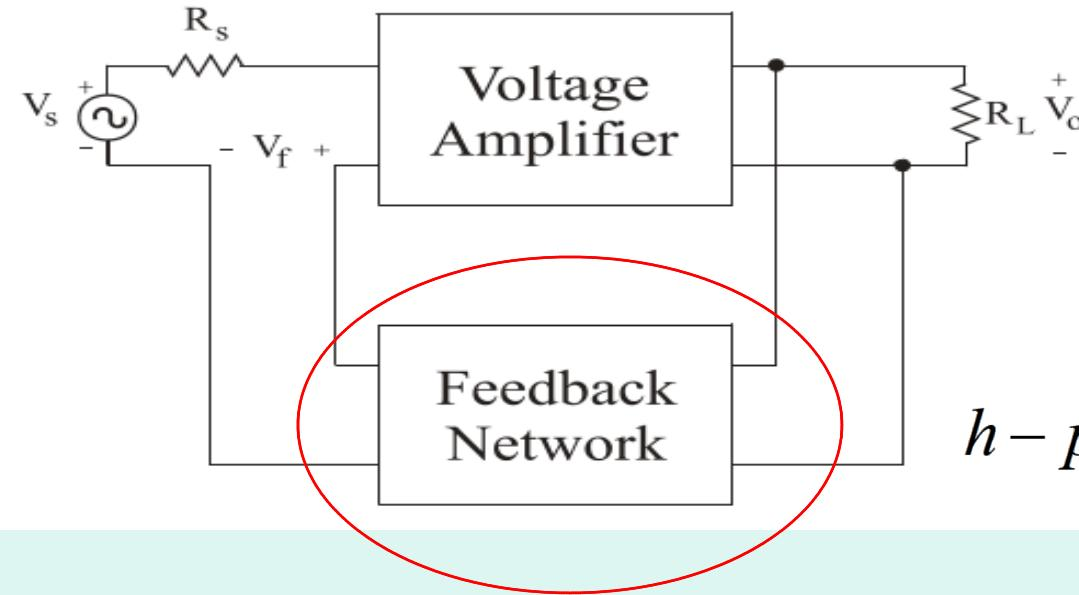
$$h - \text{parameters} : \begin{cases} V_1 = h_{11}I_1 + h_{12}V_2 \\ I_2 = h_{21}I_1 + h_{22}V_2 \end{cases}$$
