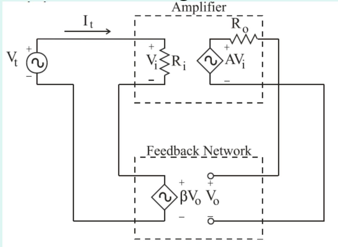
$$R_{if} = \frac{V_t}{I_t} = \frac{V_t}{\frac{V_i}{R_i}} = R_i \frac{V_i + \beta V_o}{V_i} = R_i (1 + A\beta)$$
