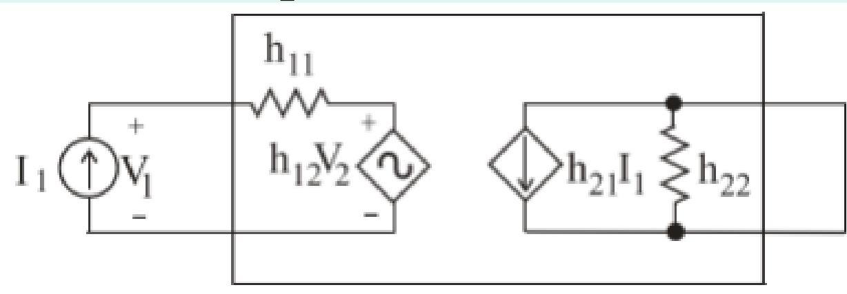
$$h_{11} = \left. \frac{V_1}{I_1} \right|_{V_2=0}$$
