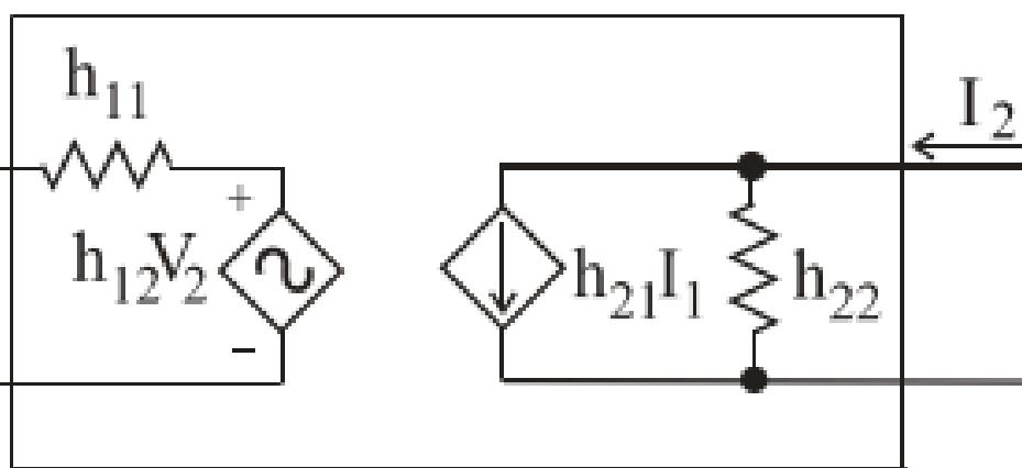
$$\begin{cases} V_1 = h_{11}I_1 + h_{12}V_2 \\ I_2 = h_{21}I_1 + h_{22}V_2 \end{cases}$$
