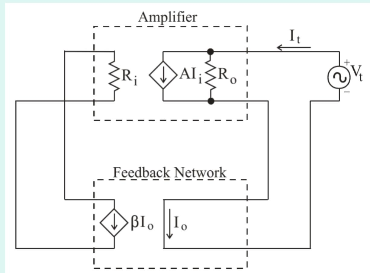
$$R_{of} = \frac{V_t}{I_t} = \frac{(I_t - AI_i)R_o}{I_t} = R_o \frac{I_t - A(-\beta I_t)}{I_t} = R_o (1 + A\beta)$$
