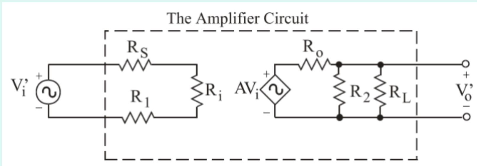
$$A' = \frac{V_o'}{V_i'} \Rightarrow A_f = \frac{A'}{1 + \beta A'} \quad R_{if} = R_i' (1 + \beta A')$$
