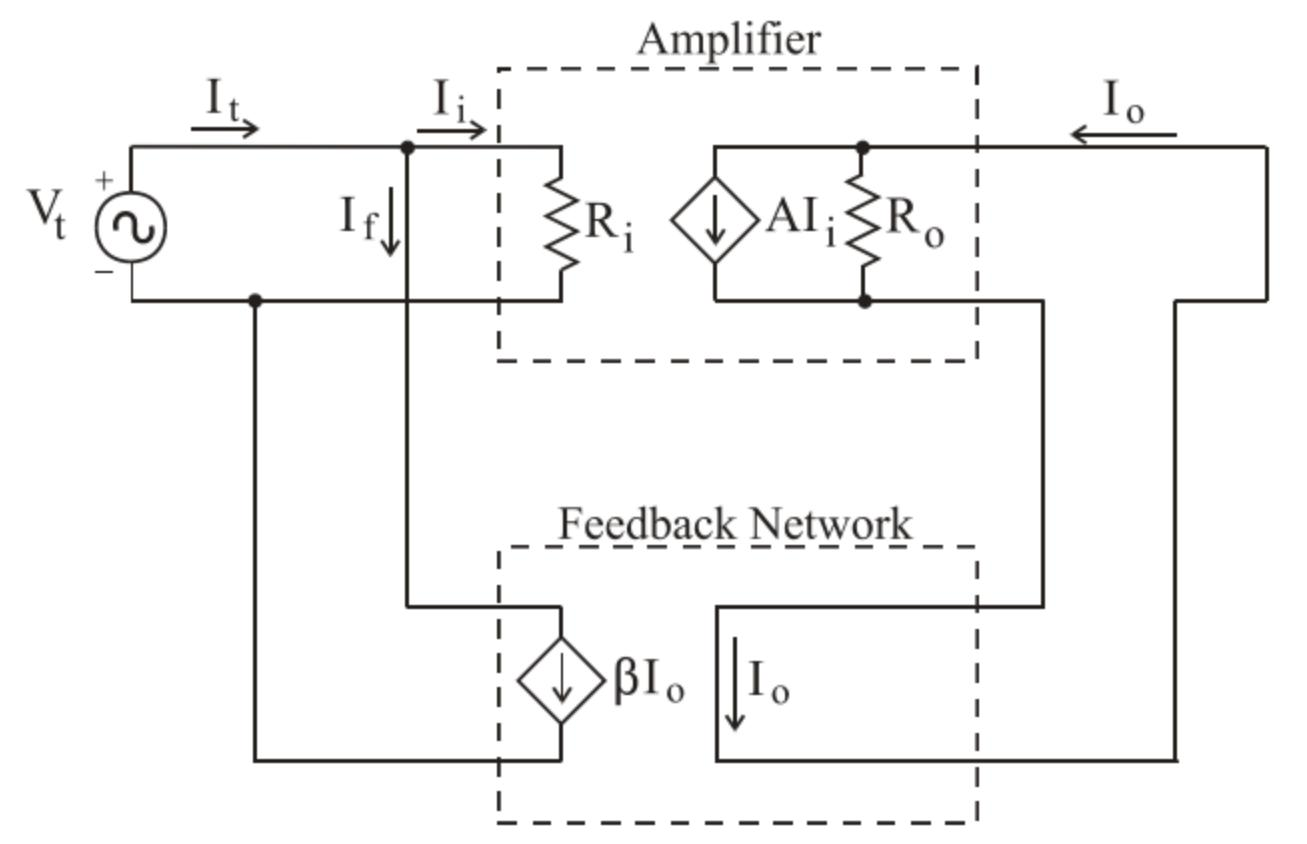
$$R_{if} = \frac{V_t}{I_t} = \frac{V_t}{\frac{V_t}{R_i} + \beta I_o} = \frac{V_t}{\frac{V_t}{R_i} + A\beta I_i} = \frac{R_i}{1 + A\beta}$$
