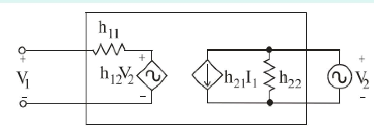
$$h_{12} = \left. \frac{V_1}{V_2} \right|_{I_1=0}$$
