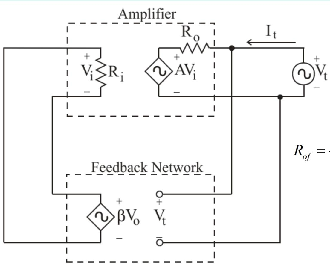
$$R_{of} = \frac{V_t}{I_t} = \frac{V_t}{\frac{V_t - AV_i}{R_o}} = R_o \frac{V_t}{V_t + A\beta V_t} = \frac{R_o}{1 + A\beta}$$
