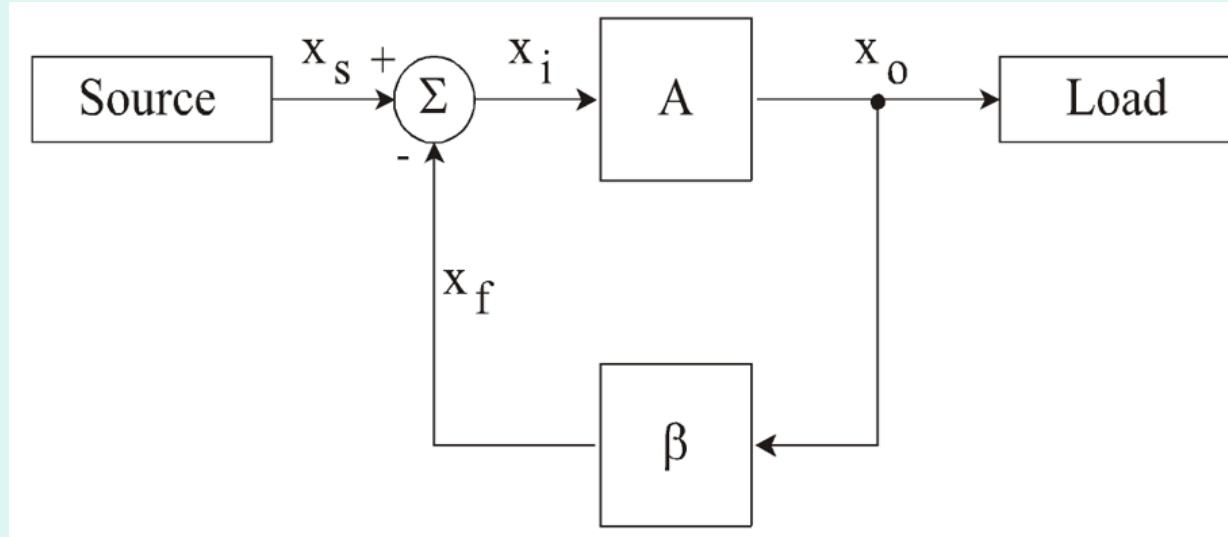
$$A_f(j\omega) = \frac{A(j\omega)}{1 + A(j\omega)\beta(j\omega)} \xrightarrow{A(j\omega)\beta(j\omega) \rightarrow -1} (A_f(j\omega) \rightarrow \infty)$$
