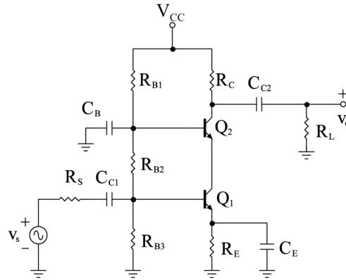
Introduce the circuit schematics into your Spice simulator software, using the 2N3904 model for the transistors. The minimum specifications for this amplifier are presented below:
