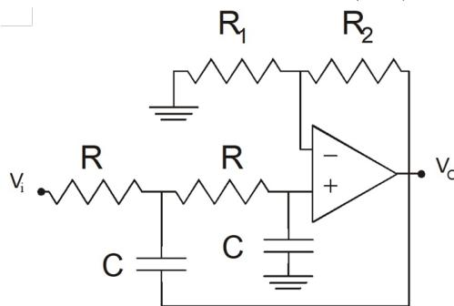
Here,  $A_M$  is the pass-band gain (and also the DC gain), given by  $A_M=1+R_2/R_1$ . The transfer function has two poles. By varying  $A_M$ , you can also control the damping ratio, so that the two poles can be made complex. This low-pass filter can be made into a 2<sup>nd</sup> order Butterworth filter by placing the poles at specific locations on a circle, centered at the origin in the s-plane.
