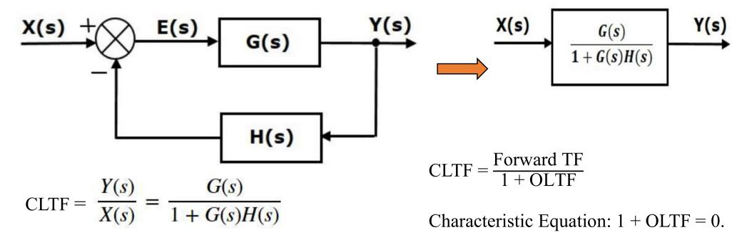
• 1 + G(s)H(s) = 0 is called the **Characteristic Equation**. It is the left hand side of this equation that we have shown by Q(s) in the previous slides. That is, Q(s) = 1 + G(s)H(s). Here, Q(s) is called the **characteristic polynomial**.
