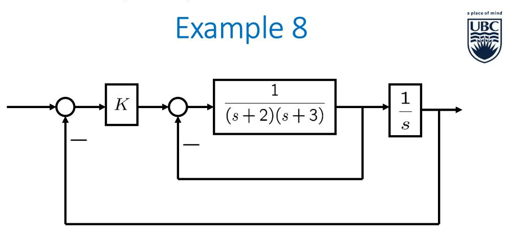
• Determine the range of *K* that stabilizes the closed-loop system.
