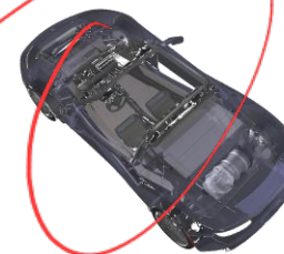
Tesla Roadster, Induction Motor, reaches 200 kW
