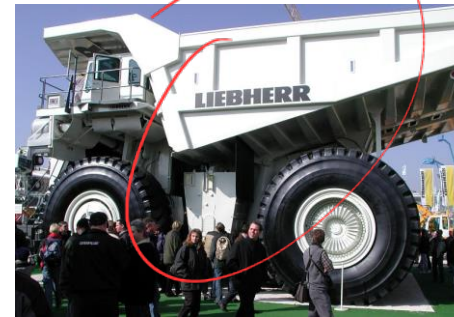
Liebherr T282B earth-hauling truck 2.7MW AC Propulsion
