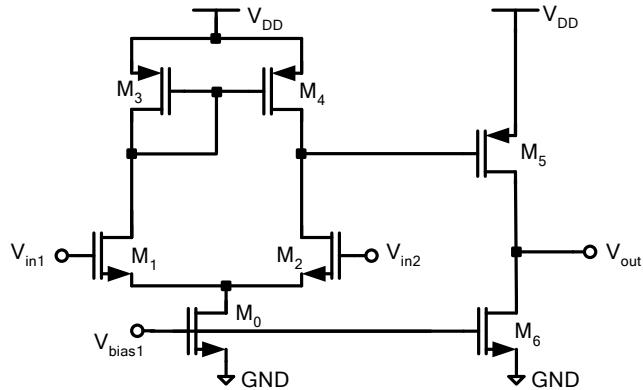
$$I_o = 0.5 \text{ mA} \Rightarrow 0.5 = \frac{1}{2} \mu_n C_{ox} \left( \frac{W}{L} \right)_o \left( V_{bias} - V_{thp} \right)^2 = \frac{1}{2} 1 \left( \frac{W}{L} \right)_o (0.7 - 0.5)^2$$
