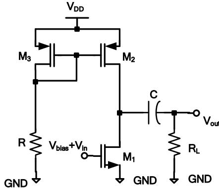
a) Assuming that the magnitude of the small-signal gain (magnitude of  $V_{out}/V_{in}$ ) is 40 V/V find  $V_{bias}$  and  $(W/L)_1$  [14 marks]
