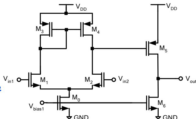
To find  $W_1$  and  $W_2$  we can use the information given about the gain and find  $g_{m1} (= g_{m2})$  and from  $g_{m1}$  and  $I_{D1}$
