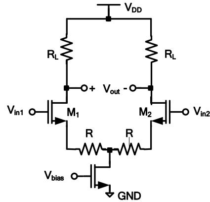
Assume all transistors are operating in saturation region and  $\lambda=\gamma=0$ ,  $V_{DD}=3$  V,  $V_{TH(NMOS)}=0.5$  V,  $\mu_nC_{ox}=1$  mA/V<sup>2</sup>,  $R=100$   $\Omega$ ,  $(W/L)_1=(W/L)_2=16$  and  $(W/L)_0=32$ . Also, assume that the  $V_{bias}=0.75$  V and the circuit is symmetric.
