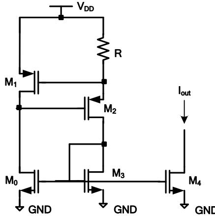
Assume all transistors are operating in saturation region and  $\lambda=\gamma=0$ ,  $V_{DD}=3$  V,  $V_{TH(NMOS)}=0.5$  V,  $V_{TH(PMOS)}= -0.5$  V,  $\mu_n C_{ox}=200 \mu\text{A/V}^2$ , and  $\mu_p C_{ox}=100 \mu\text{A/V}^2$ . Also, assume that  $M_0$ ,  $M_3$  and  $M_4$  have the same aspect ratio.
