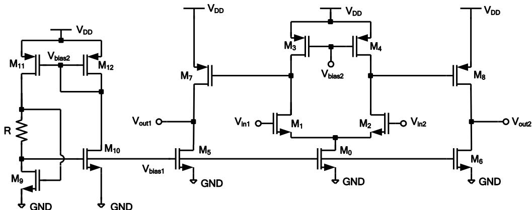
Use the following design specifications (Note that the gate of  $M_{12}$  is also connected to the gate of  $M_3$ ):
