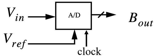
$$V_{ref}(b_1 2^{-1} + b_2 2^{-2} + \dots + b_N 2^{-N}) = V_{in} \pm x$$
