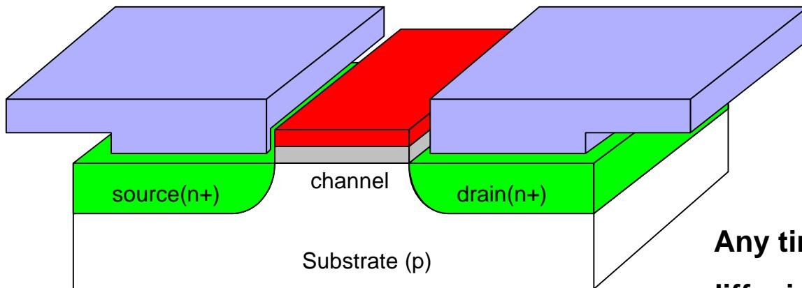
**Any time polysilicon crosses diffusion, we have a transistor**
