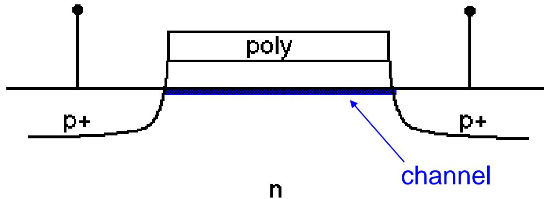
Channel carriers have + charge. Attracted by a negative voltage
