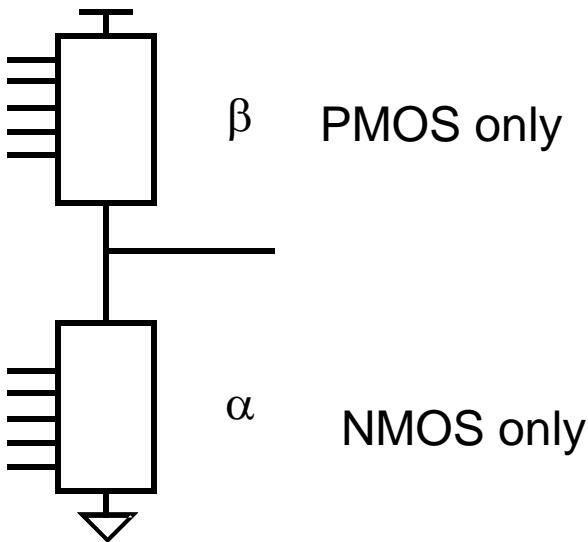
The pulldown network connects the output to  $Gnd$  when  $f$  is true.
