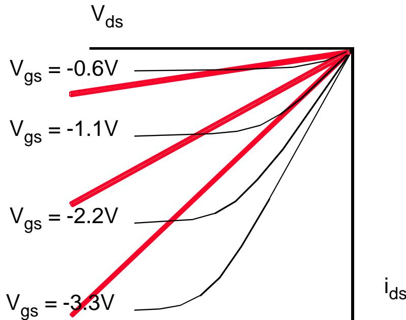
Again we will use a voltage variable resistor approximation for timing calc.
