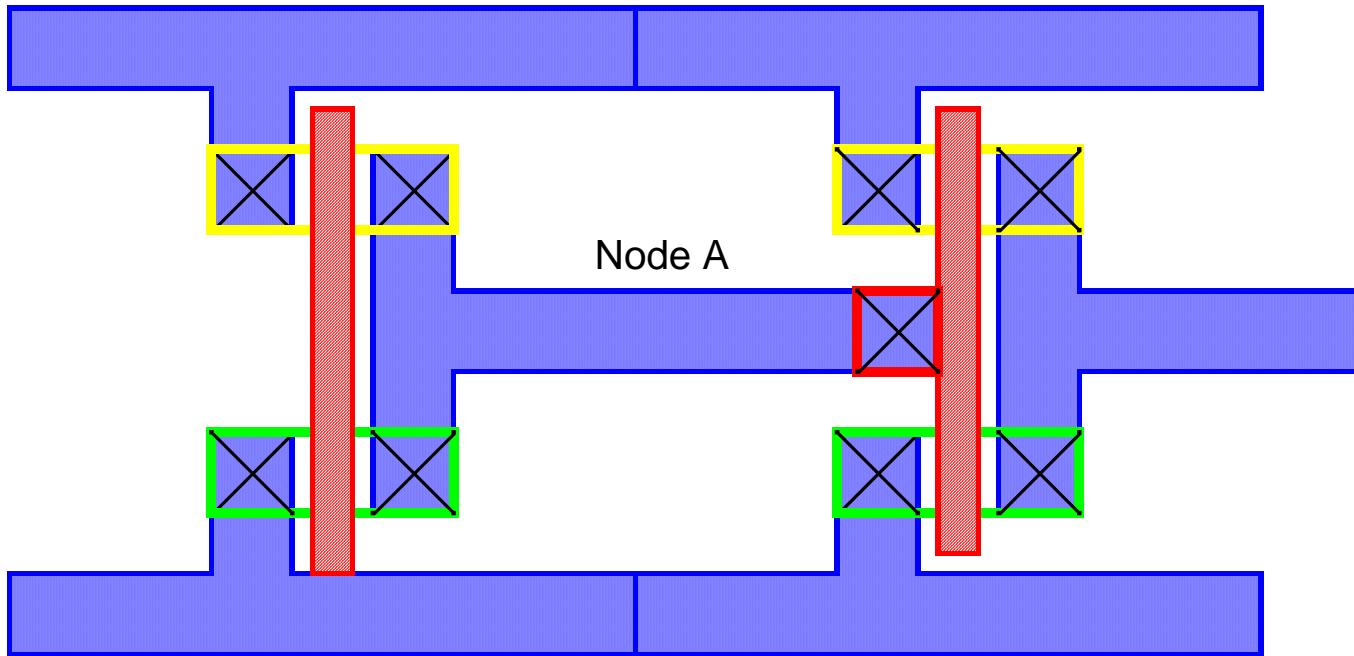
Node A: 2 diffusion regions each  $2\mu$  ( $4\lambda$ ), 2 gate regions each  $2\mu$ ,  $16\mu$  Metal 1 (12 $\lambda$  vertical, 20 $\lambda$  horizontal), 14 $\lambda$  poly=  $2*2\mu*2fF/\mu + 2*2\mu*2fF/\mu + 16\mu*0.3fF/\mu + 7\mu*0.2fF/\mu = 8fF + 8fF + 4.8fF + 1.4fF = 22.2fF$
