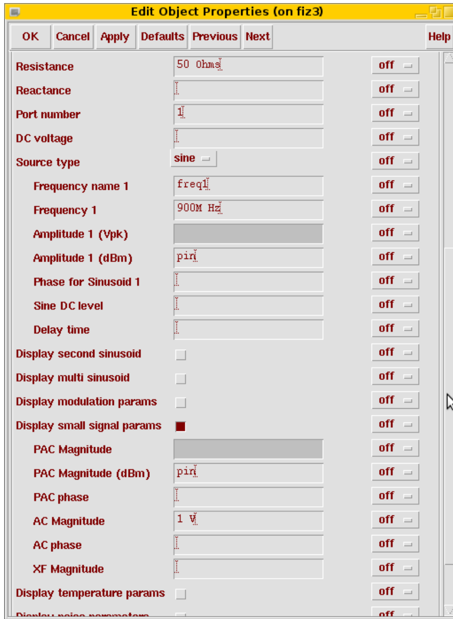
Fig. 14: Modifying the input port for pss+pac analysis
