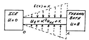
FIGURE 1. Bar subject to a time-independent heat source distributed along its length with inhomogeneous Dirichlet BC
