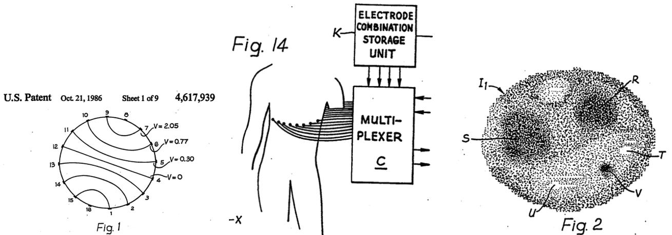
(a) Level sets of potential field used in the US Patent (b) Medical imaging device (c) Actual image obtained from EIT
