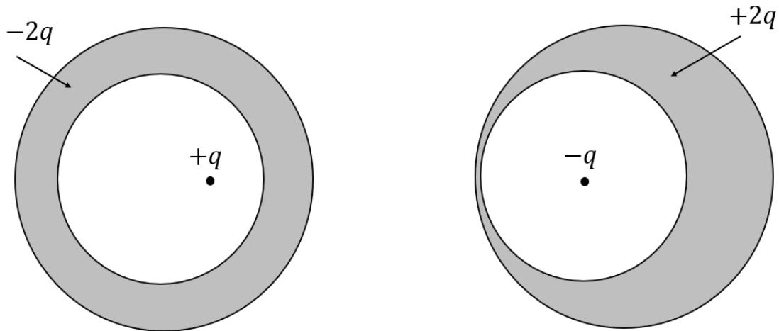
**Problem 2 [12 pts].** A dielectric spherical shell is charged with a negative surface charge density,  $-\sigma$ , on its inner surface. In addition, a point charge  $+2q$  is fixed at the center of the cavity in the middle of the shell, and  $2q = 2(4\pi a^2)|\sigma|$ . The outer surface of the shell is uncharged. The dielectric is linear with a dielectric permittivity  $\epsilon$ . The inner radius of the shell is  $a$ , the outer radius is  $b$ .
