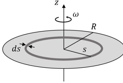
The loop shown in the figure at a distance  $s$  from the center of the disk carries current
