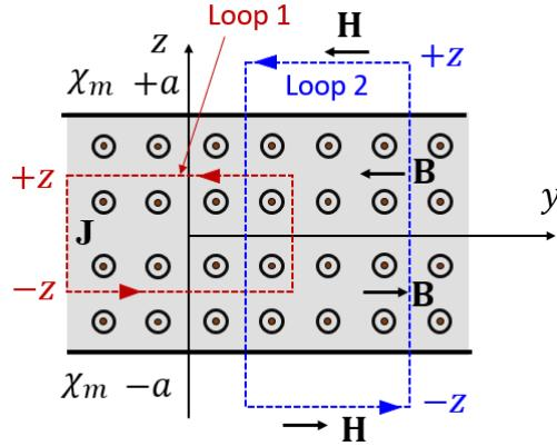
Outside the slab, we will have magnetization, so we should be more careful when choosing what to start with. We will use Ampere's law for auxiliary field  $\mathbf{H}$ , since we know the free current,  $\mathbf{J}_f = \mathbf{J}$ . Using Loop 2 with width  $L_2$  form the figure we get:
