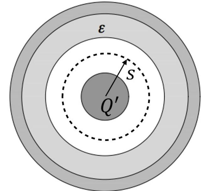
$$\rightarrow \Delta V = \frac{Q'}{2\pi} \left( \frac{1}{\epsilon_0} \ln(b/a) + \frac{1}{\epsilon} \ln(d/b) \right) \quad C' = \frac{Q'}{\Delta V}$$
