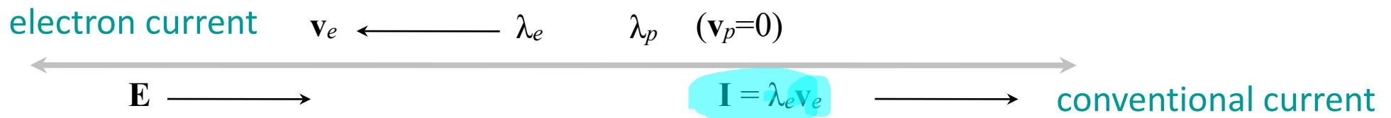
The motion of  $\lambda_e$  generates a steady current:  $I = |\lambda|v$ . This has unit of charge per unit time, i.e.  $[I] = [\Delta q/\Delta t]$ , which is the amount of charge passing a given point on the wire per unit time. Note that the wire **remains neutral**.
