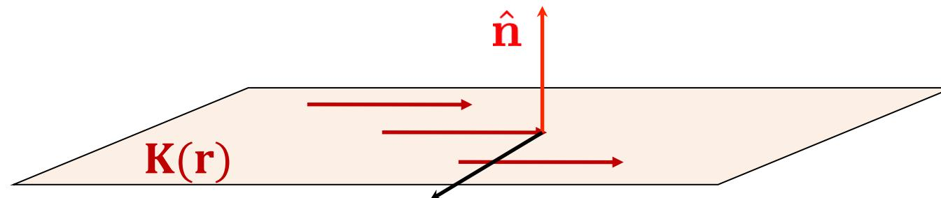
Think of the surface current as a bunch of parallel wires running along the surface, each carrying a current. Each wire contributes a bit of magnetic field that circulates around it per the right hand rule. This produces some (extra)  $\mathbf{B}$  into the page below the surface and out of the page above it => surface current creates a jump in  $\mathbf{B}_{\parallel}$
