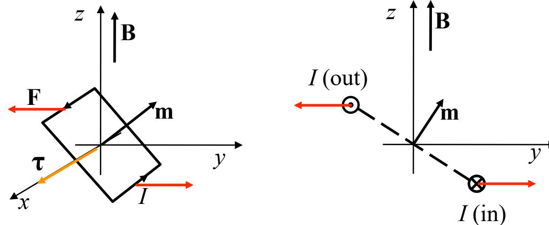
The magnetic torque on  $\mathbf{m}$  has the same form as for the electric dipole,  $\mathbf{p}$ :  $\tau_m = \mathbf{m} \times \mathbf{B}$
