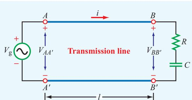
**Figure 2-2** Generator connected to an RC circuit through a transmission line of length  $l$ .
