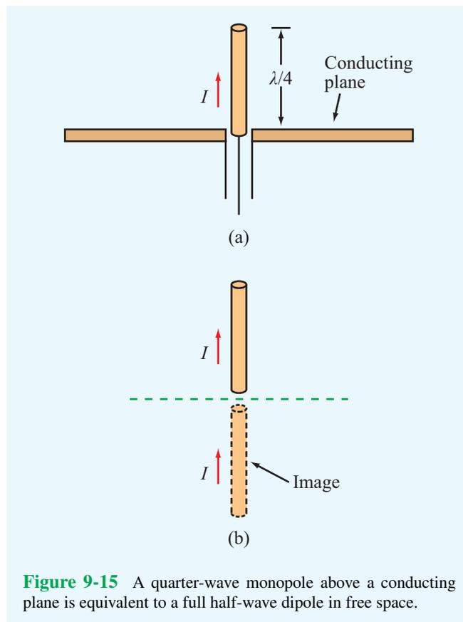
**Figure 9-15** A quarter-wave monopole above a conducting plane is equivalent to a full half-wave dipole in free space.
