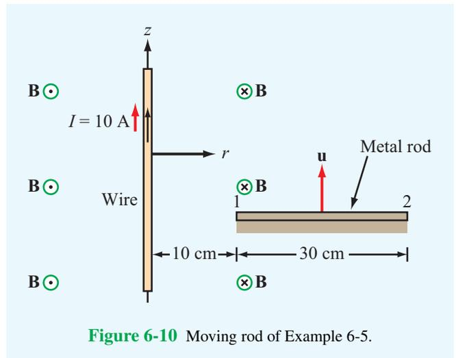
**Figure 6-10** Moving rod of Example 6-5.
