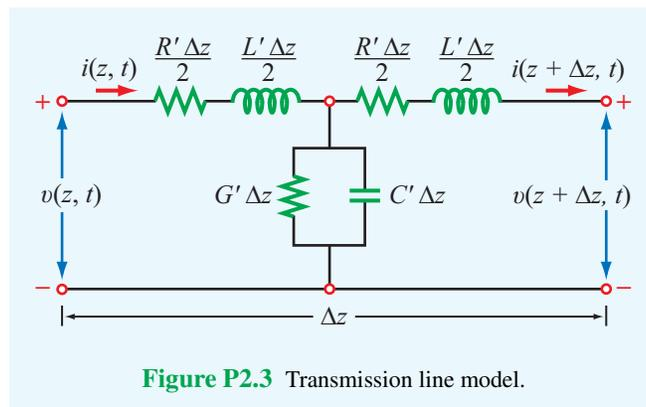
Figure P2.3 Transmission line model.
