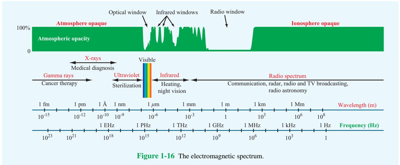
Figure 1-16 The electromagnetic spectrum.
