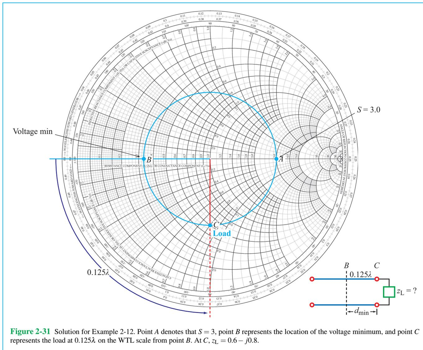
**Figure 2-31** Solution for Example 2-12. Point A denotes that  $S = 3$ , point B represents the location of the voltage minimum, and point C represents the load at  $0.125\lambda$  on the WTL scale from point B. At C,  $z_L = 0.6 - j0.8$ .
