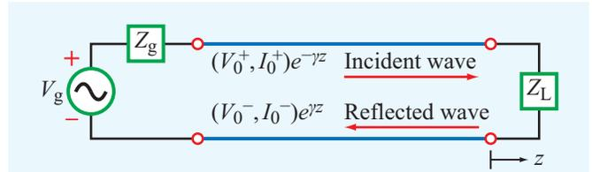
**Figure 2-9** In general, a transmission line can support two traveling waves: an incident wave (with voltage and current amplitudes  $(V_0^+, I_0^+)$ ) traveling along the  $+z$  direction (towards the load) and a reflected wave (with  $(V_0^-, I_0^-)$ ) traveling along the  $-z$  direction (towards the source).
