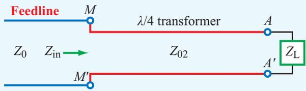
(a) If  $Z_L$  is real: in-series  $\lambda/4$  transformer inserted at  $AA'$
