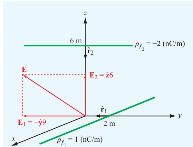
**Figure 4-11** Two infinite lines of charge (Example 4-7).
