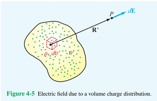
**Figure 4-5** Electric field due to a volume charge distribution.
