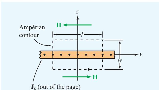
**Figure 5-19** A thin current sheet in the  $x$ - $y$  plane carrying a surface current density  $\mathbf{J}_s = \hat{\mathbf{x}}J_s$  (Example 5-6).
