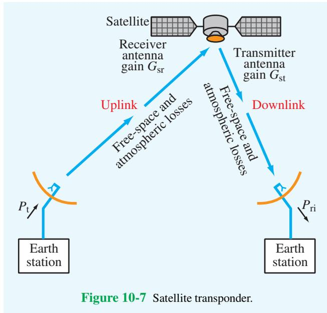
**Figure 10-7** Satellite transponder.
