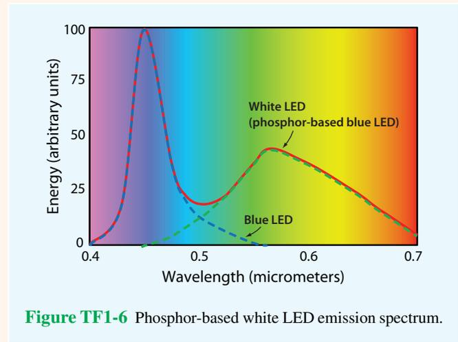
With the blue LED/phosphor conversion technique, a blue LED is used with phosphor powder particles suspended in the epoxy resin that encapsulates it. The blue light emitted by the LED is absorbed by the phosphor particles and then reemitted as a broad spectrum (**Fig. TF1-6**). To generate high-intensity light, several LEDs are clustered into a single enclosure.
