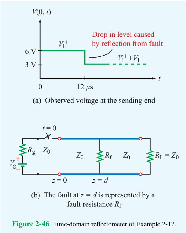
**Figure 2-46** Time-domain reflectometer of Example 2-17.
