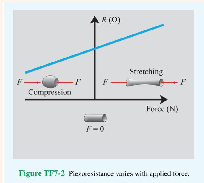
**Figure TF7-2** Piezoresistance varies with applied force.
