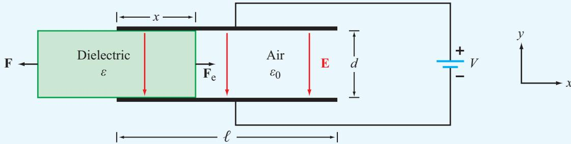
**Figure 4-29** Parallel-plate capacitor with slidable dielectric block.
