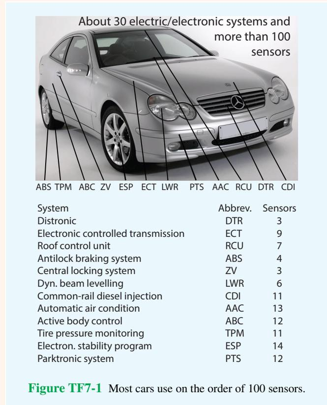
**Figure TF7-1** Most cars use on the order of 100 sensors.
