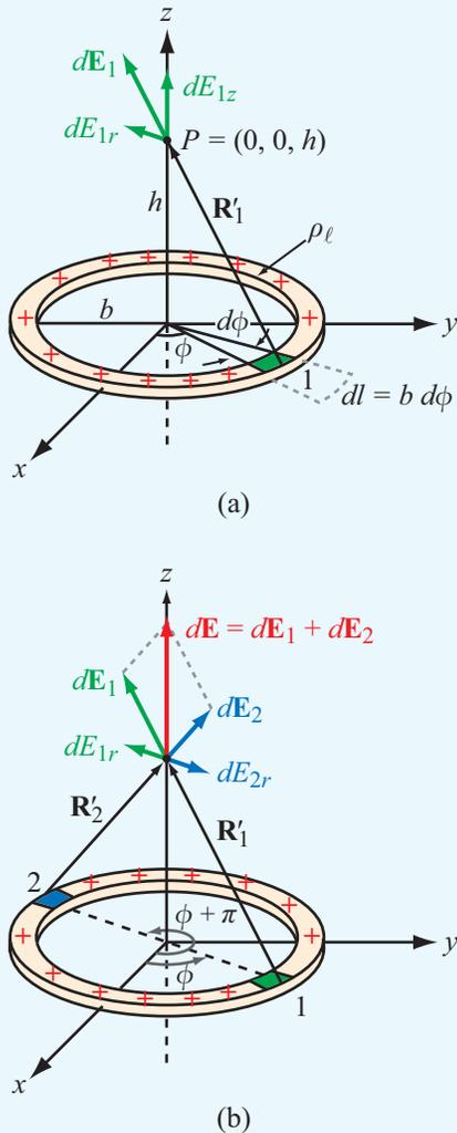
**Figure 4-6** Ring of charge with line density  $\rho_\ell$ . (a) The field  $d\mathbf{E}_1$  due to infinitesimal segment 1 and (b) the fields  $d\mathbf{E}_1$  and  $d\mathbf{E}_2$  due to segments at diametrically opposite locations (Example 4-4).
