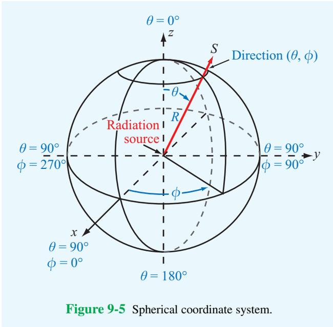
Figure 9-5 Spherical coordinate system.
