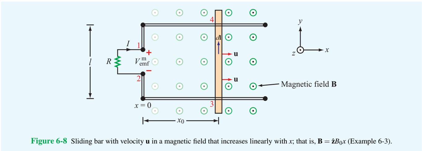
**Figure 6-8** Sliding bar with velocity  $\mathbf{u}$  in a magnetic field that increases linearly with  $x$ ; that is,  $\mathbf{B} = \hat{\mathbf{z}}B_0x$  (Example 6-3).
