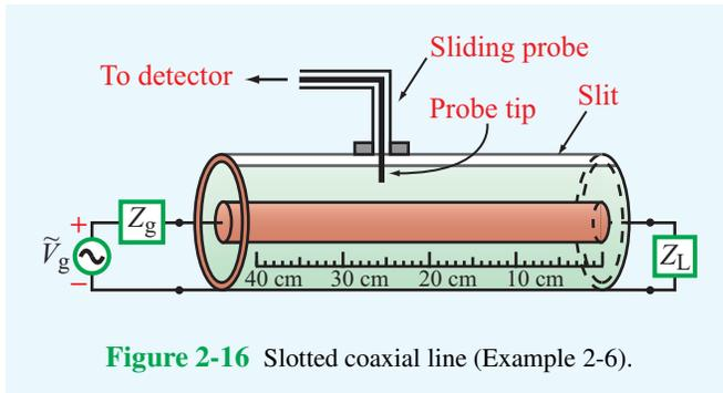
Figure 2-16 Slotted coaxial line (Example 2-6).
