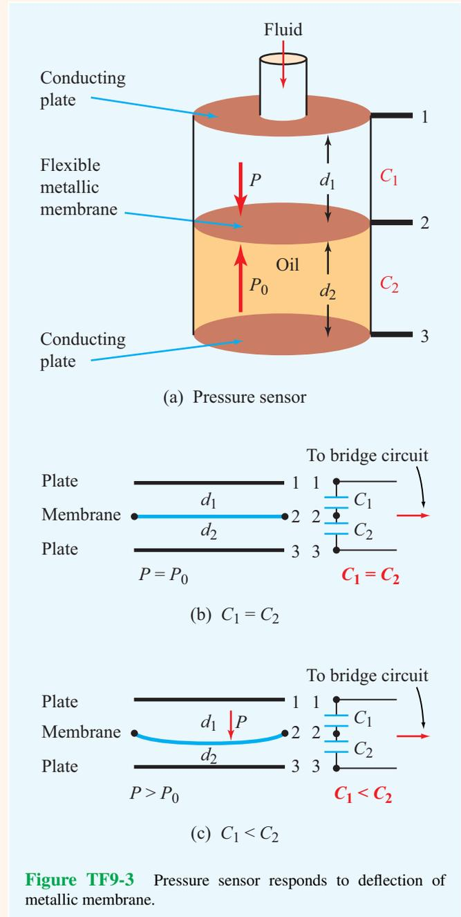
**Figure TF9-3** Pressure sensor responds to deflection of metallic membrane.
