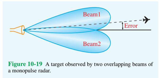
**Figure 10-19** A target observed by two overlapping beams of a monopulse radar.
