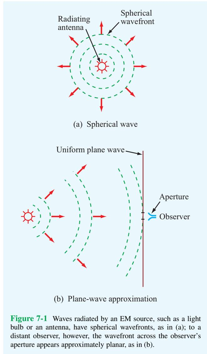
**Figure 7-1** Waves radiated by an EM source, such as a light bulb or an antenna, have spherical wavefronts, as in (a); to a distant observer, however, the wavefront across the observer's aperture appears approximately planar, as in (b).
