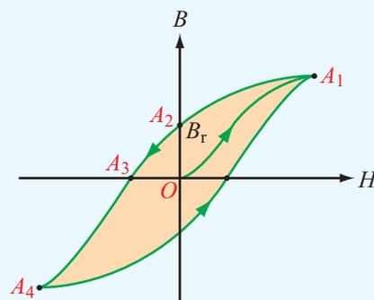
**Figure 5-22** Typical hysteresis curve for a ferromagnetic material.
