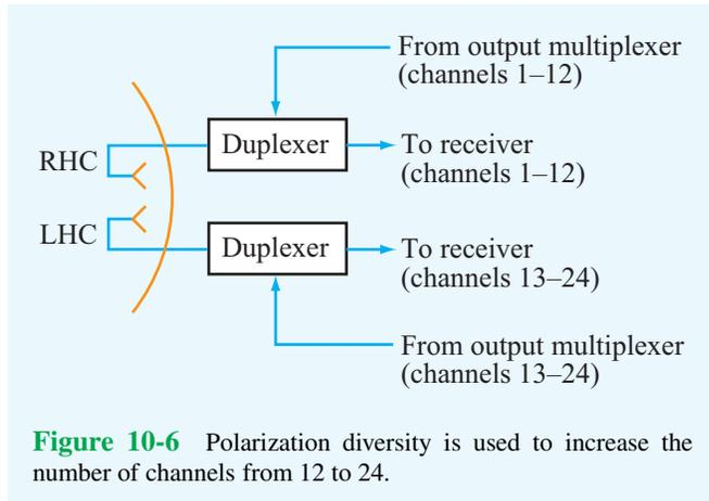
**Figure 10-6** Polarization diversity is used to increase the number of channels from 12 to 24.
