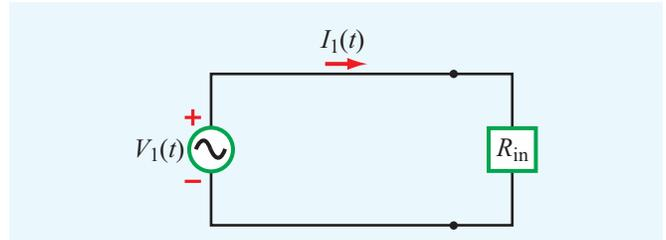
Figure 6-6 Equivalent circuit for the primary side of the transformer.
