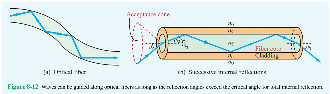
**Figure 8-12** Waves can be guided along optical fibers as long as the reflection angles exceed the critical angle for total internal reflection.
