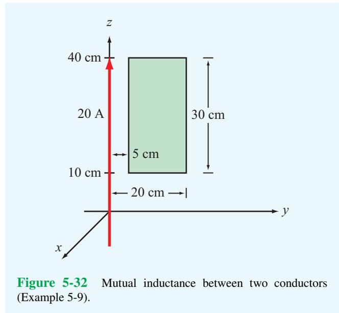
**Figure 5-32** Mutual inductance between two conductors (Example 5-9).
