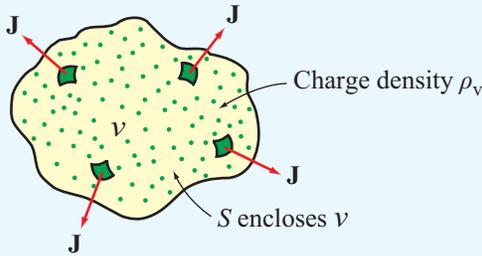
**Figure 6-14** The total current flowing out of a volume  $\mathcal{V}$  is equal to the flux of the current density  $\mathbf{J}$  through the surface  $S$ , which in turn is equal to the rate of decrease of the charge enclosed in  $\mathcal{V}$ .
