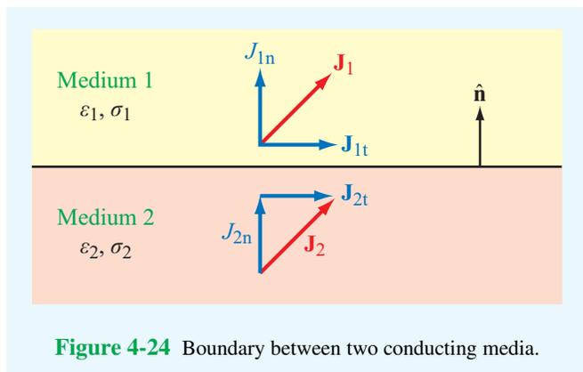
**Figure 4-24** Boundary between two conducting media.
