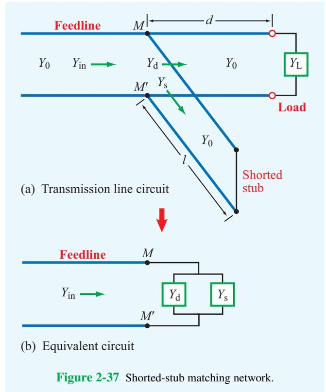
**Figure 2-37** Shorted-stub matching network.
