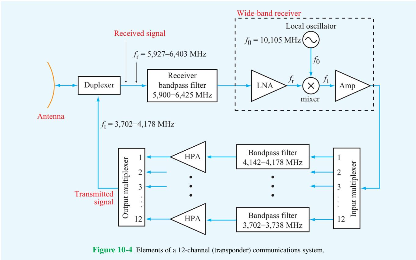
Figure 10-4 Elements of a 12-channel (transponder) communications system.
