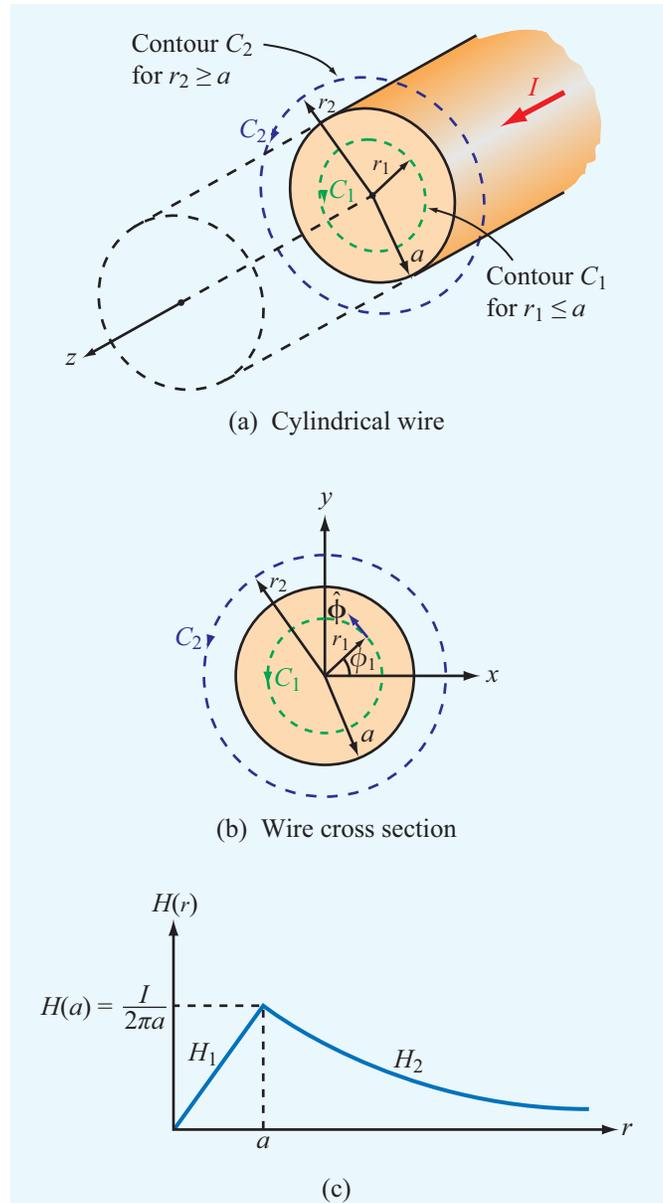
**Figure 5-17** Infinitely long wire of radius  $a$  carrying a uniform current  $I$  along the  $+z$  direction: (a) general configuration showing contours  $C_1$  and  $C_2$ ; (b) cross-sectional view; and (c) a plot of  $H$  versus  $r$  (Example 5-4).
