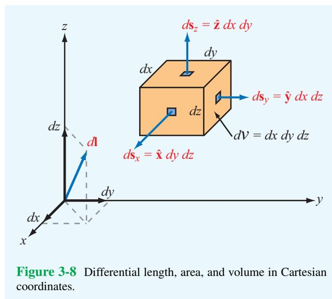
**Figure 3-8** Differential length, area, and volume in Cartesian coordinates.
