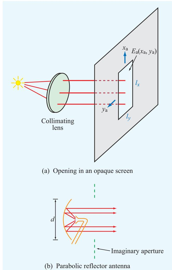
**Figure 9-21** Radiation by apertures: (a) an opening in an opaque screen illuminated by a light source through a collimating lens and (b) a parabolic dish reflector illuminated by a small horn antenna.
