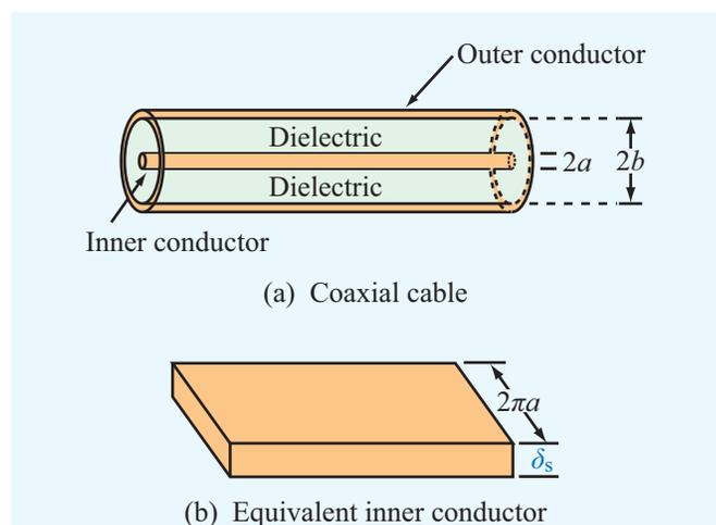
**Figure 7-16** The inner conductor of the coaxial cable in (a) is represented in (b) by a planar conductor of width  $2\pi a$  and depth  $\delta_s$ , as if its skin has been cut along its length on the bottom side and then unfurled into a planar geometry.
