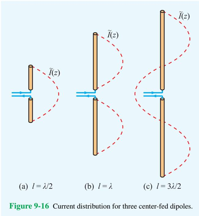
**Figure 9-16** Current distribution for three center-fed dipoles.
