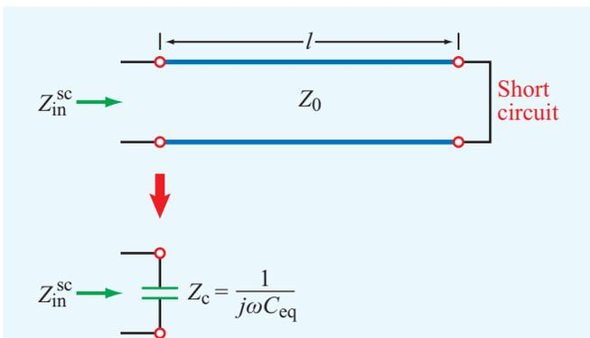
**Figure 2-20** Shorted line as an equivalent capacitor (Example 2-8).
