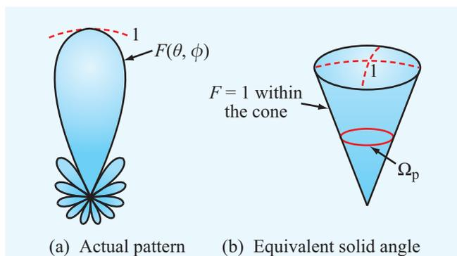
Figure 9-11 The pattern solid angle  $\Omega_p$  defines an equivalent cone over which all of the radiation of the actual antenna is concentrated with uniform intensity equal to the maximum of the actual pattern.
