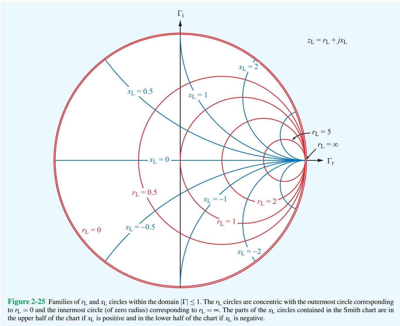
**Figure 2-25** Families of  $r_L$  and  $x_L$  circles within the domain  $|\Gamma| \leq 1$ . The  $r_L$  circles are concentric with the outermost circle corresponding to  $r_L = 0$  and the innermost circle (of zero radius) corresponding to  $r_L = \infty$ . The parts of the  $x_L$  circles contained in the Smith chart are in the upper half of the chart if  $x_L$  is positive and in the lower half of the chart if  $x_L$  is negative.
