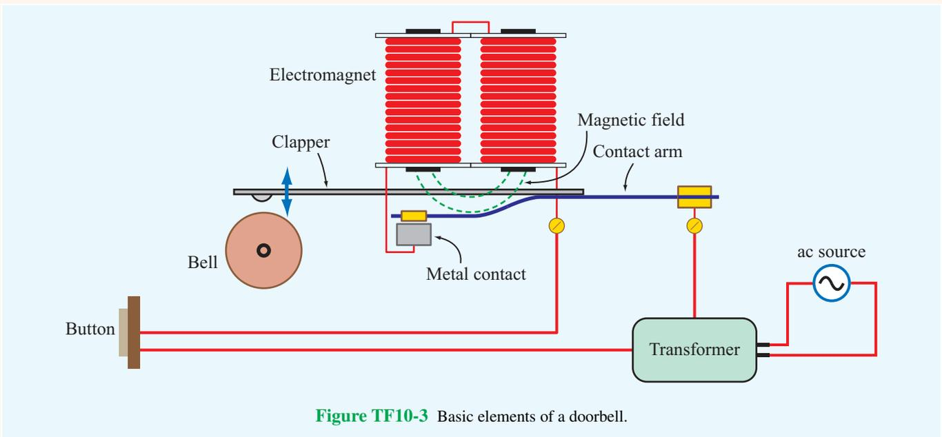
Figure TF10-3 Basic elements of a doorbell.
