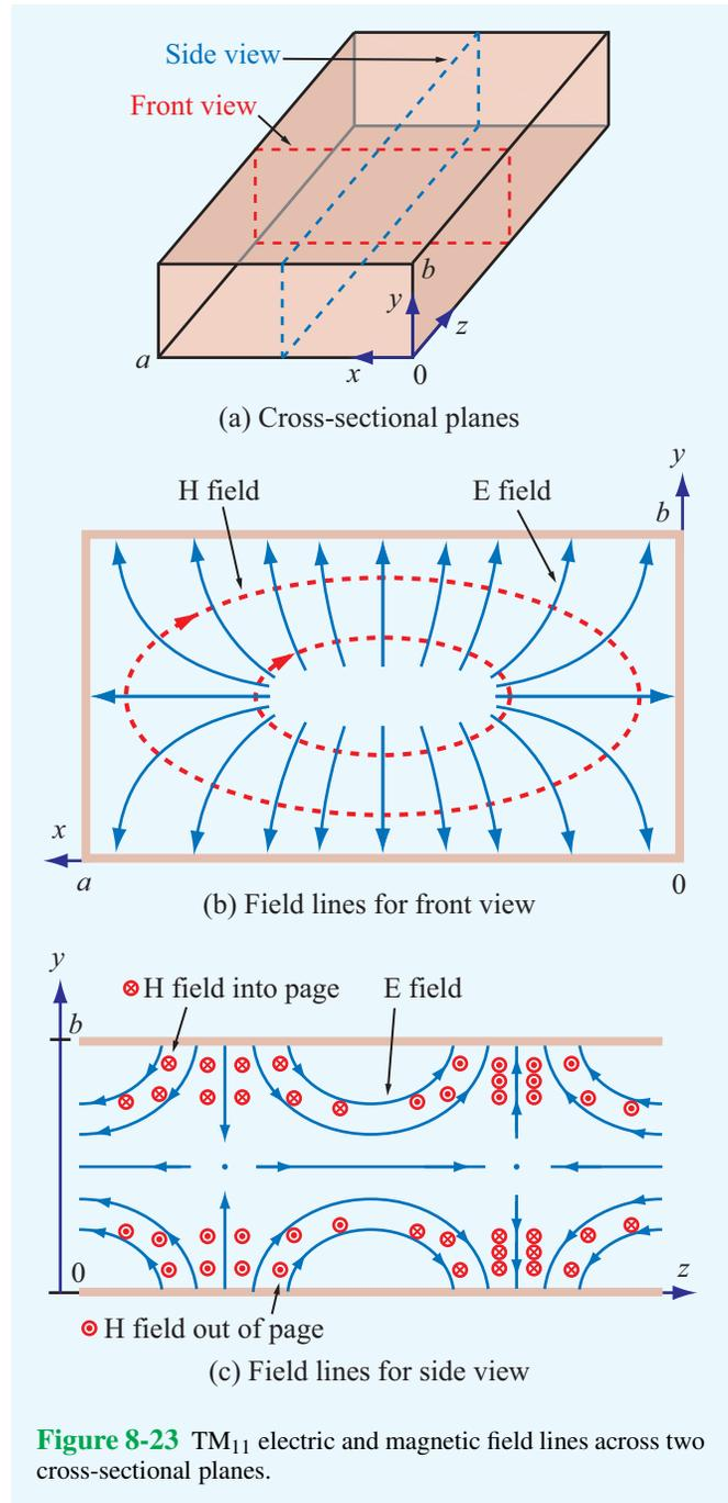
**Figure 8-23**  $TM_{11}$  electric and magnetic field lines across two cross-sectional planes.
