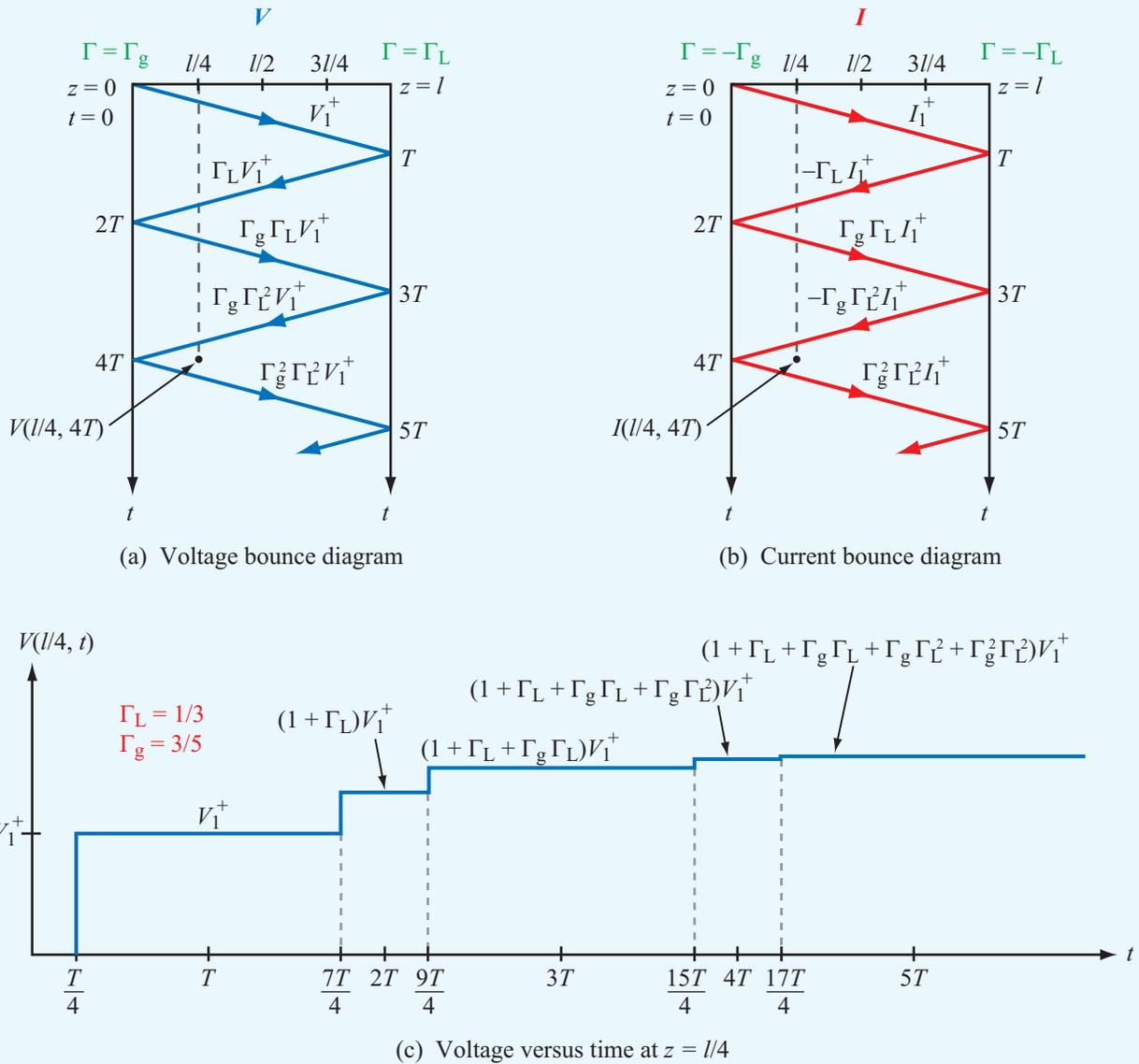
**Figure 2-44** Bounce diagrams for (a) voltage and (b) current. In (c), the voltage variation with time at  $z = l/4$  for a circuit with  $\Gamma_g = 3/5$  and  $\Gamma_L = 1/3$  is deduced from the vertical dashed line at  $l/4$  in (a).
