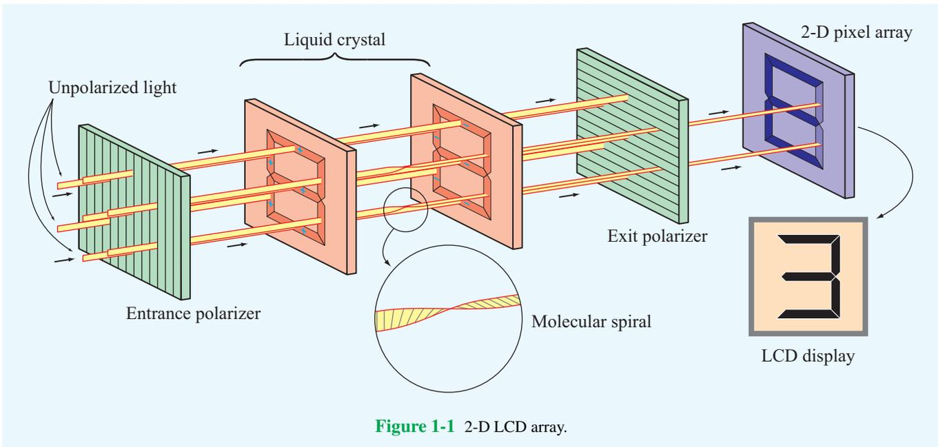
Figure 1-1 2-D LCD array.
