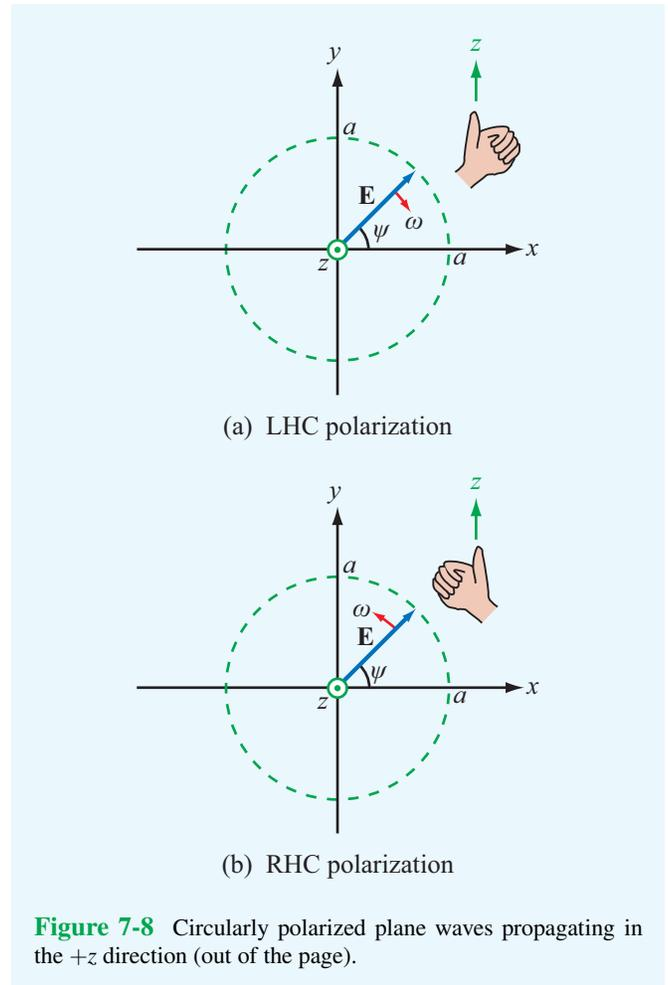
**Figure 7-8** Circularly polarized plane waves propagating in the +z direction (out of the page).
