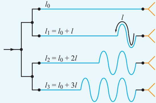
**Figure 9-34** An example of a feeding arrangement for frequency-scanning arrays.
