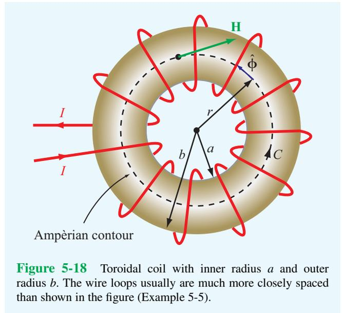
**Figure 5-18** Toroidal coil with inner radius  $a$  and outer radius  $b$ . The wire loops usually are much more closely spaced than shown in the figure (Example 5-5).
