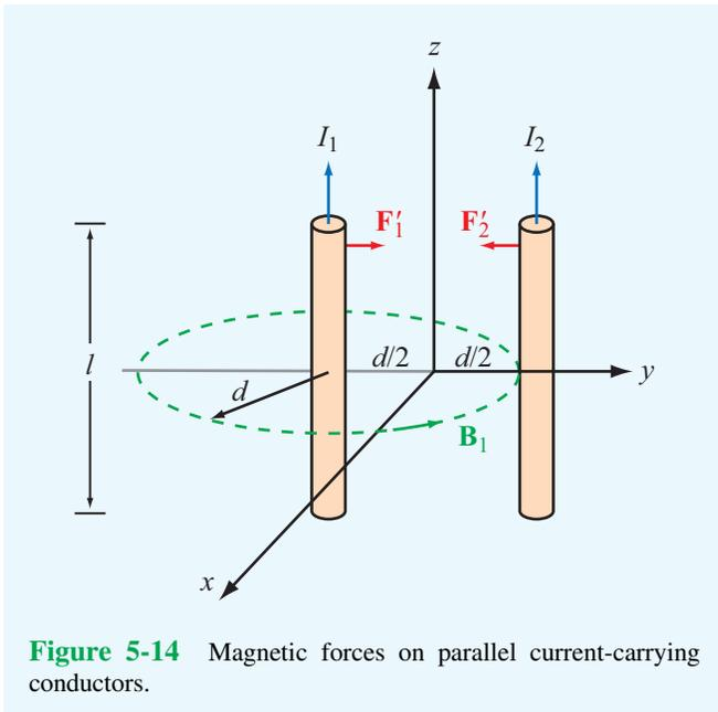
**Figure 5-14** Magnetic forces on parallel current-carrying conductors.
