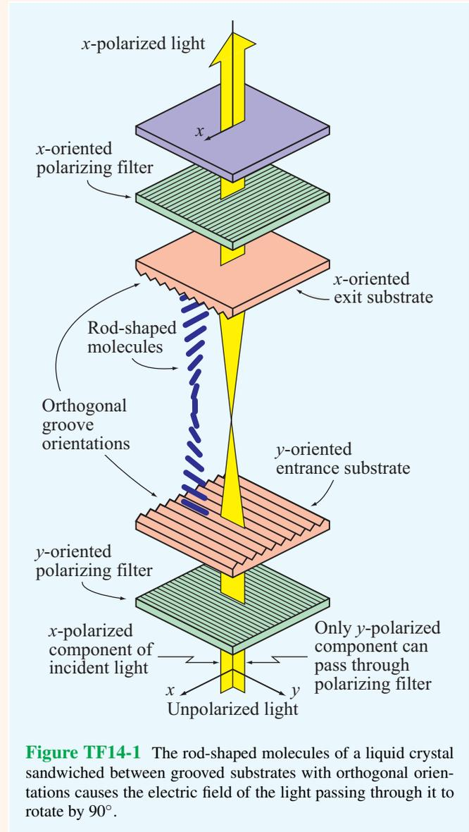
**Figure TF14-1** The rod-shaped molecules of a liquid crystal sandwiched between grooved substrates with orthogonal orientations causes the electric field of the light passing through it to rotate by  $90^\circ$ .
