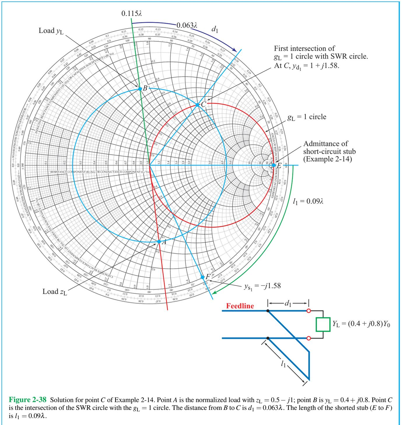
**Figure 2-38** Solution for point C of Example 2-14. Point A is the normalized load with  $z_L = 0.5 - j1$ ; point B is  $y_L = 0.4 + j0.8$ . Point C is the intersection of the SWR circle with the  $g_L = 1$  circle. The distance from B to C is  $d_1 = 0.063\lambda$ . The length of the shorted stub (E to F) is  $l_1 = 0.09\lambda$ .
