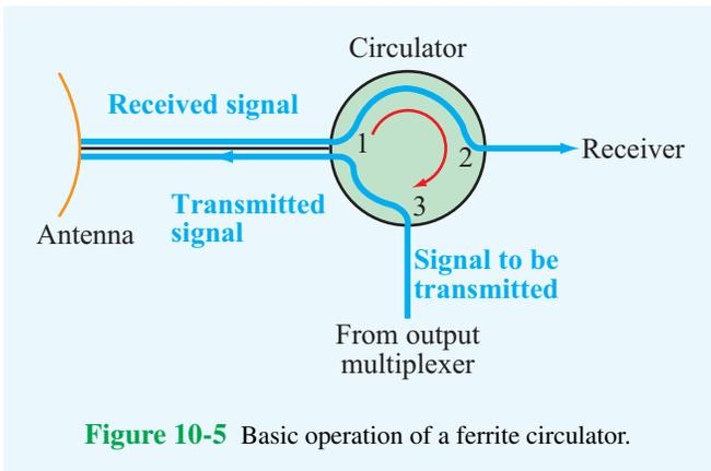
Figure 10-5 Basic operation of a ferrite circulator.
