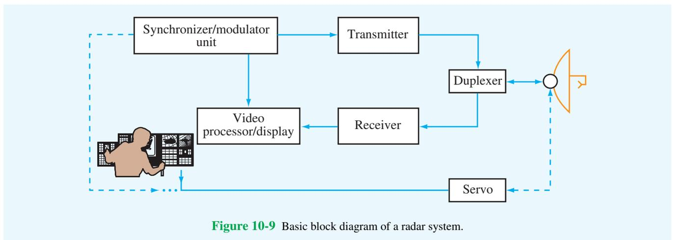
**Figure 10-9** Basic block diagram of a radar system.
