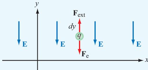
**Figure 4-12** Work done in moving a charge  $q$  a distance  $dy$  against the electric field  $\mathbf{E}$  is  $dW = qE dy$ .
