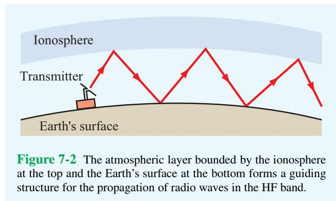
**Figure 7-2** The atmospheric layer bounded by the ionosphere at the top and the Earth's surface at the bottom forms a guiding structure for the propagation of radio waves in the HF band.
