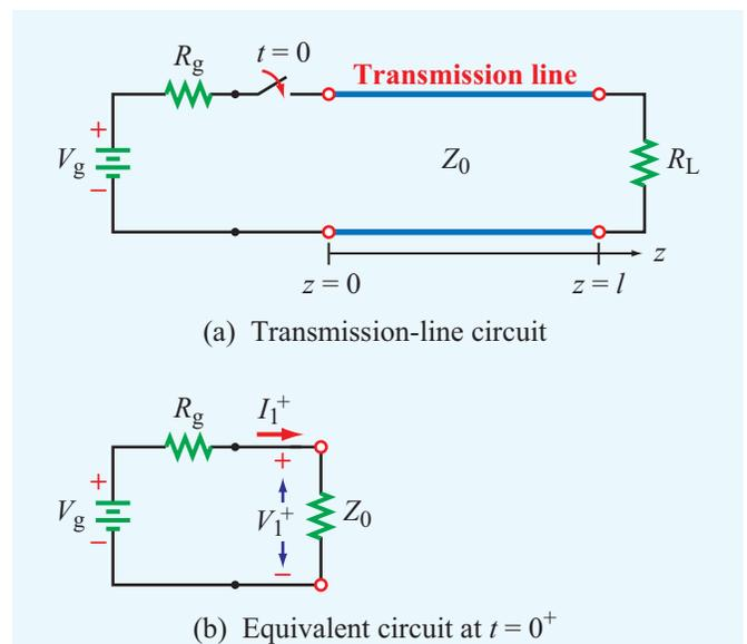
**Figure 2-42** At  $t = 0^+$ , immediately after closing the switch in the circuit in part (a), the circuit can be represented by the equivalent circuit in part (b). This is because from that instant and until a reflection is received back from the load the generator circuit “sees” only an impedance  $Z_0$ .
