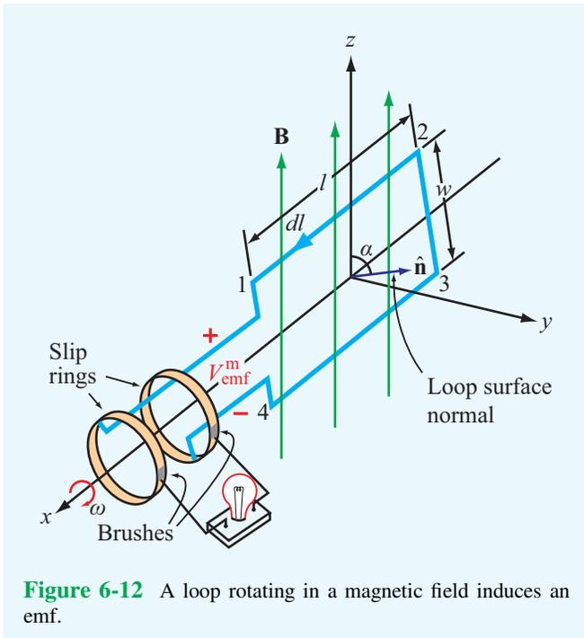
**Figure 6-12** A loop rotating in a magnetic field induces an emf.
