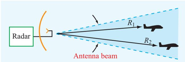
**Figure 10-11** Radar beam viewing two targets at ranges  $R_1$  and  $R_2$ .
