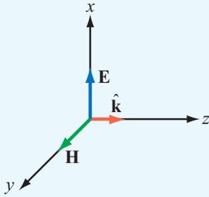
**Figure 7-4** A transverse electromagnetic (TEM) wave propagating in the direction  $\hat{\mathbf{k}} = \hat{\mathbf{z}}$ . For all TEM waves,  $\hat{\mathbf{k}}$  is parallel to  $\mathbf{E} \times \mathbf{H}$ .
