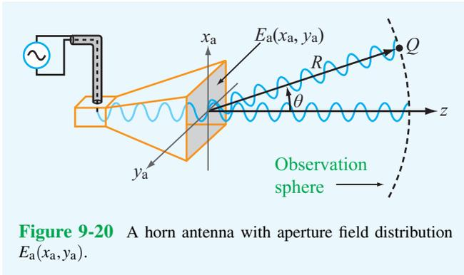
**Figure 9-20** A horn antenna with aperture field distribution  $E_a(x_a, y_a)$ .
