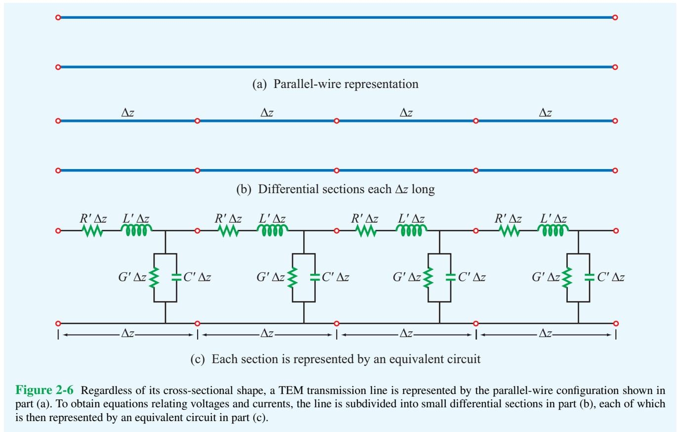
each of these lines, the expressions are functions of two sets of parameters: (1) geometric parameters defining the cross-sectional dimensions of the given line and (2) the electromagnetic constitutive parameters of the conducting and insulating materials. The pertinent geometric parameters are:
