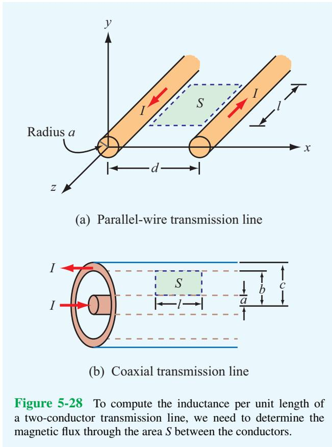
**Figure 5-28** To compute the inductance per unit length of a two-conductor transmission line, we need to determine the magnetic flux through the area  $S$  between the conductors.
