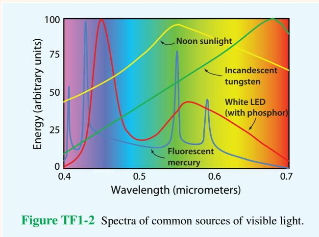
Figure TF1-2 Spectra of common sources of visible light.
