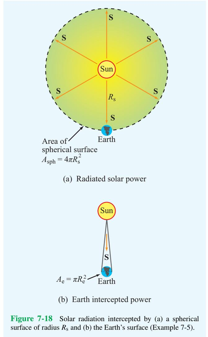
**Figure 7-18** Solar radiation intercepted by (a) a spherical surface of radius  $R_s$  and (b) the Earth's surface (Example 7-5).
