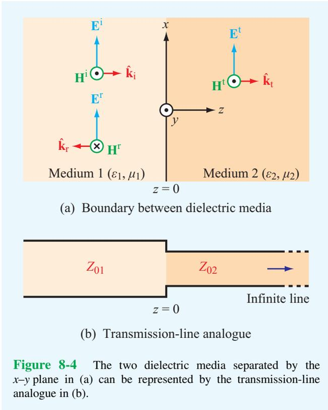
**Figure 8-4** The two dielectric media separated by the  $x$ - $y$  plane in (a) can be represented by the transmission-line analogue in (b).
