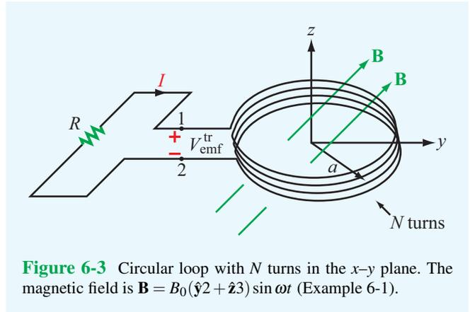
**Figure 6-3** Circular loop with  $N$  turns in the  $x$ - $y$  plane. The magnetic field is  $\mathbf{B} = B_0(\hat{y}2 + \hat{z}3) \sin \omega t$  (Example 6-1).
