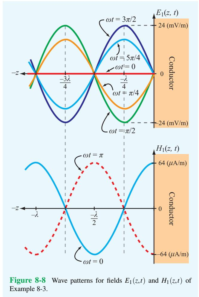
**Figure 8-8** Wave patterns for fields  $E_1(z, t)$  and  $H_1(z, t)$  of Example 8-3.
