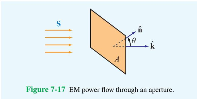
Figure 7-17 EM power flow through an aperture.
