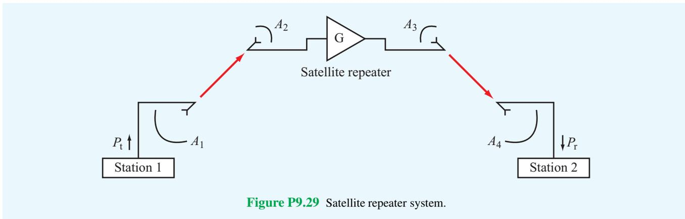
Figure P9.29 Satellite repeater system.
