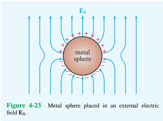
**Figure 4-23** Metal sphere placed in an external electric field  $\mathbf{E}_0$ .
