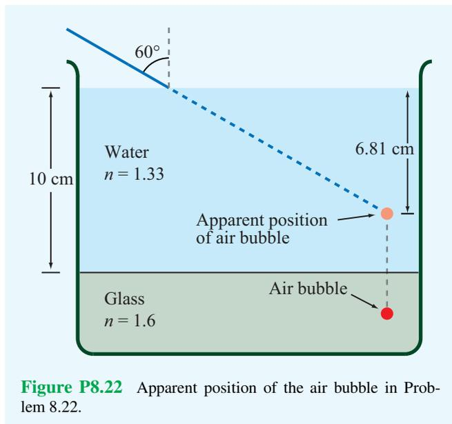
**Figure P8.22** Apparent position of the air bubble in Problem 8.22.
