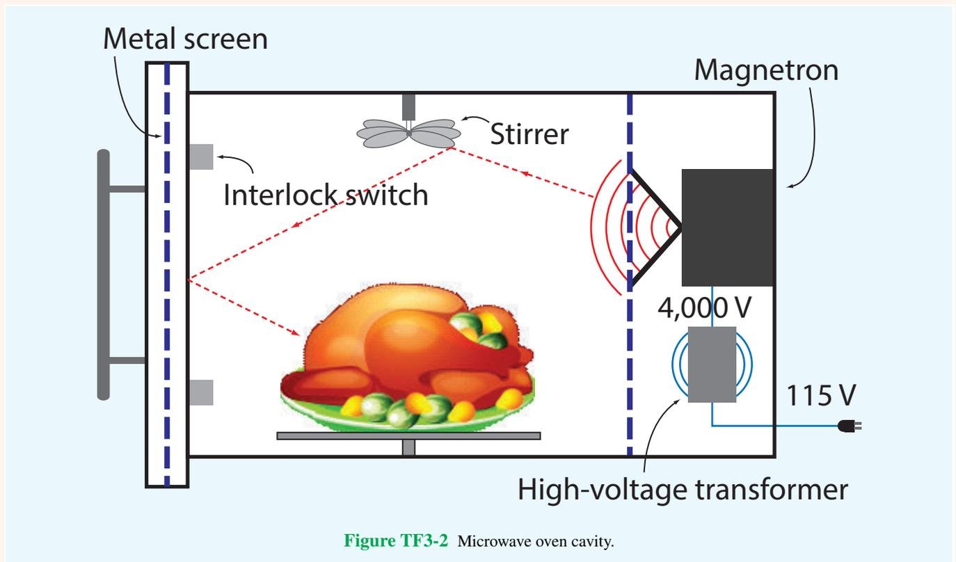
Figure TF3-2 Microwave oven cavity.
