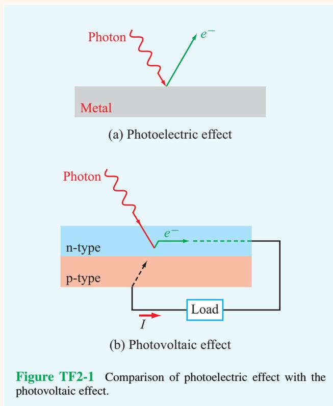
**Figure TF2-1** Comparison of photoelectric effect with the photovoltaic effect.
