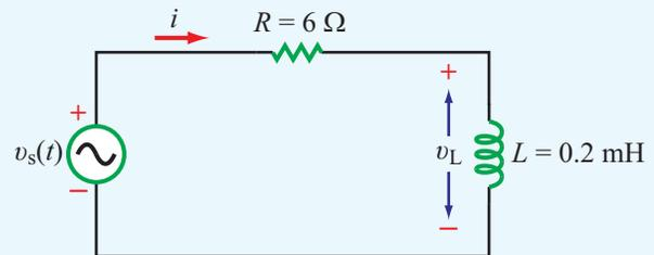
**Figure 1-21** RL circuit (Example 1-4).
