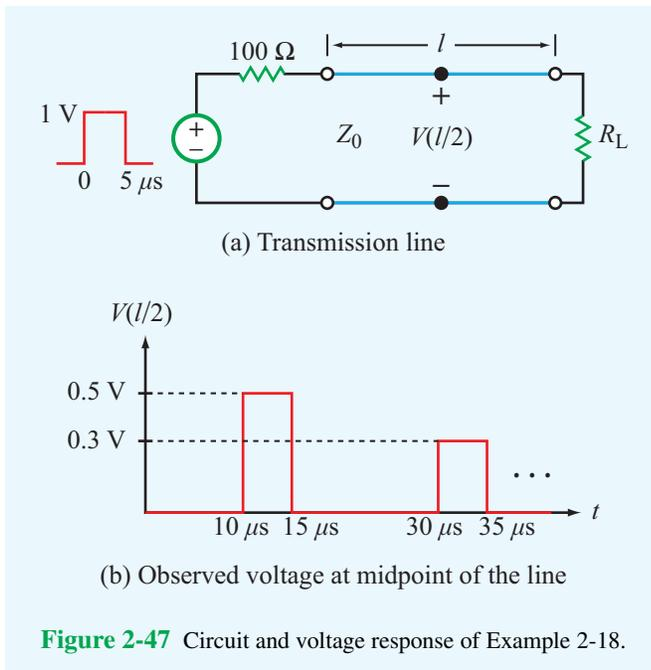
**Figure 2-47** Circuit and voltage response of Example 2-18.
