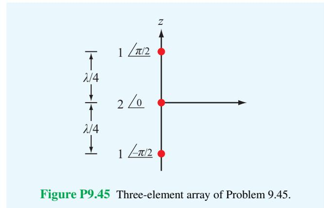
**Figure P9.45** Three-element array of Problem 9.45.
