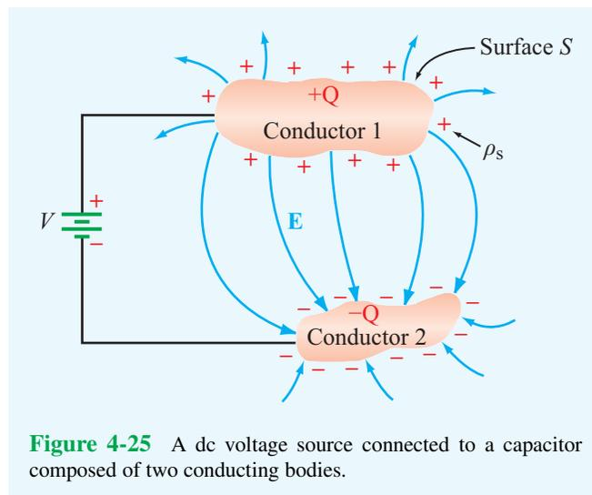
**Figure 4-25** A dc voltage source connected to a capacitor composed of two conducting bodies.
