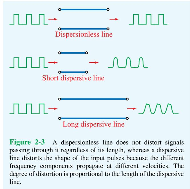
**Figure 2-3** A dispersionless line does not distort signals passing through it regardless of its length, whereas a dispersive line distorts the shape of the input pulses because the different frequency components propagate at different velocities. The degree of distortion is proportional to the length of the dispersive line.
