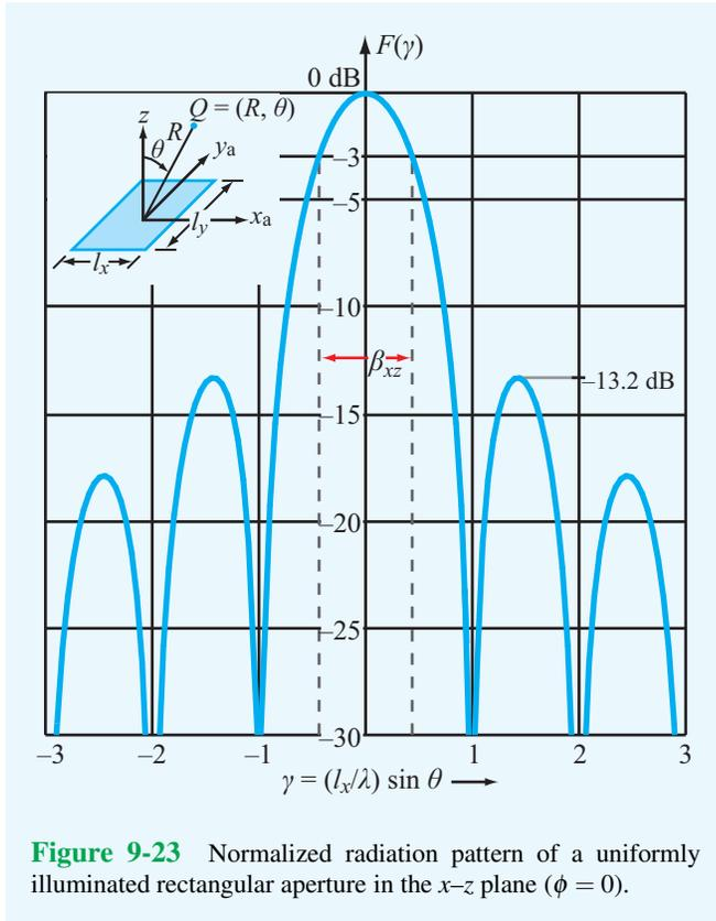
**Figure 9-23** Normalized radiation pattern of a uniformly illuminated rectangular aperture in the  $x$ - $z$  plane ( $\phi = 0$ ).
