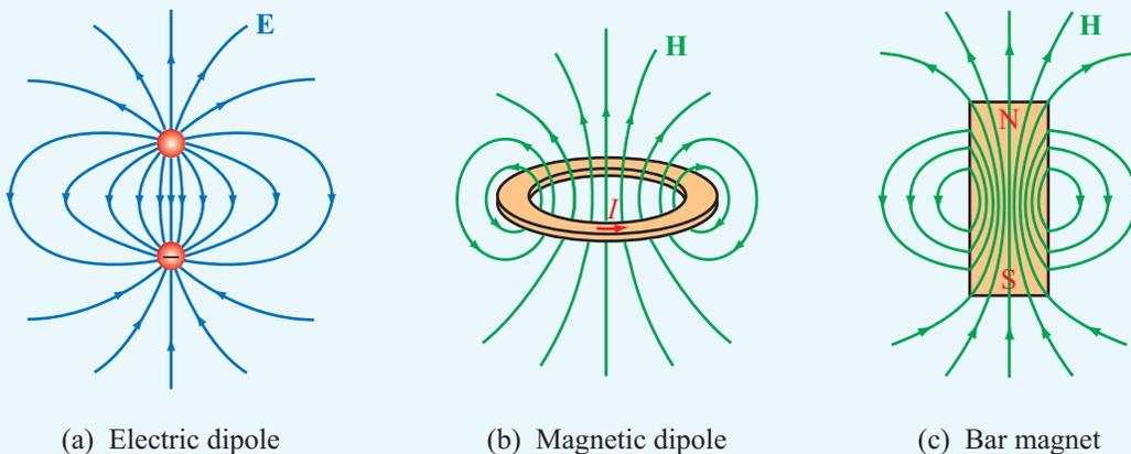
**Figure 5-13** Patterns of (a) the electric field of an electric dipole, (b) the magnetic field of a magnetic dipole, and (c) the magnetic field of a bar magnet. Far away from the sources, the field patterns are similar in all three cases.
