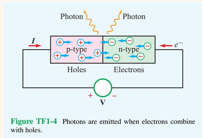
Figure TF1-4 Photons are emitted when electrons combine with holes.
