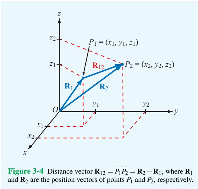
**Figure 3-4** Distance vector  $\mathbf{R}_{12} = \overrightarrow{P_1P_2} = \mathbf{R}_2 - \mathbf{R}_1$ , where  $\mathbf{R}_1$  and  $\mathbf{R}_2$  are the position vectors of points  $P_1$  and  $P_2$ , respectively.
