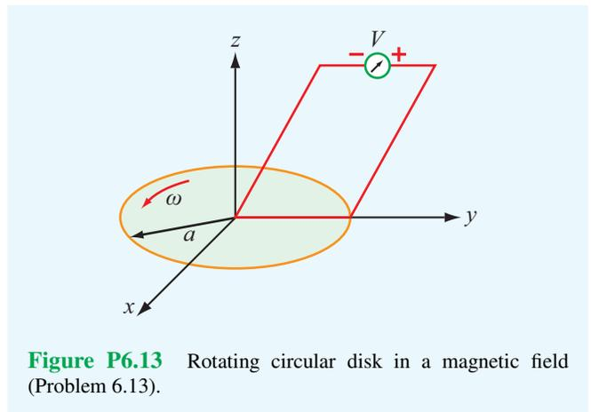
Figure P6.13 Rotating circular disk in a magnetic field (Problem 6.13).
