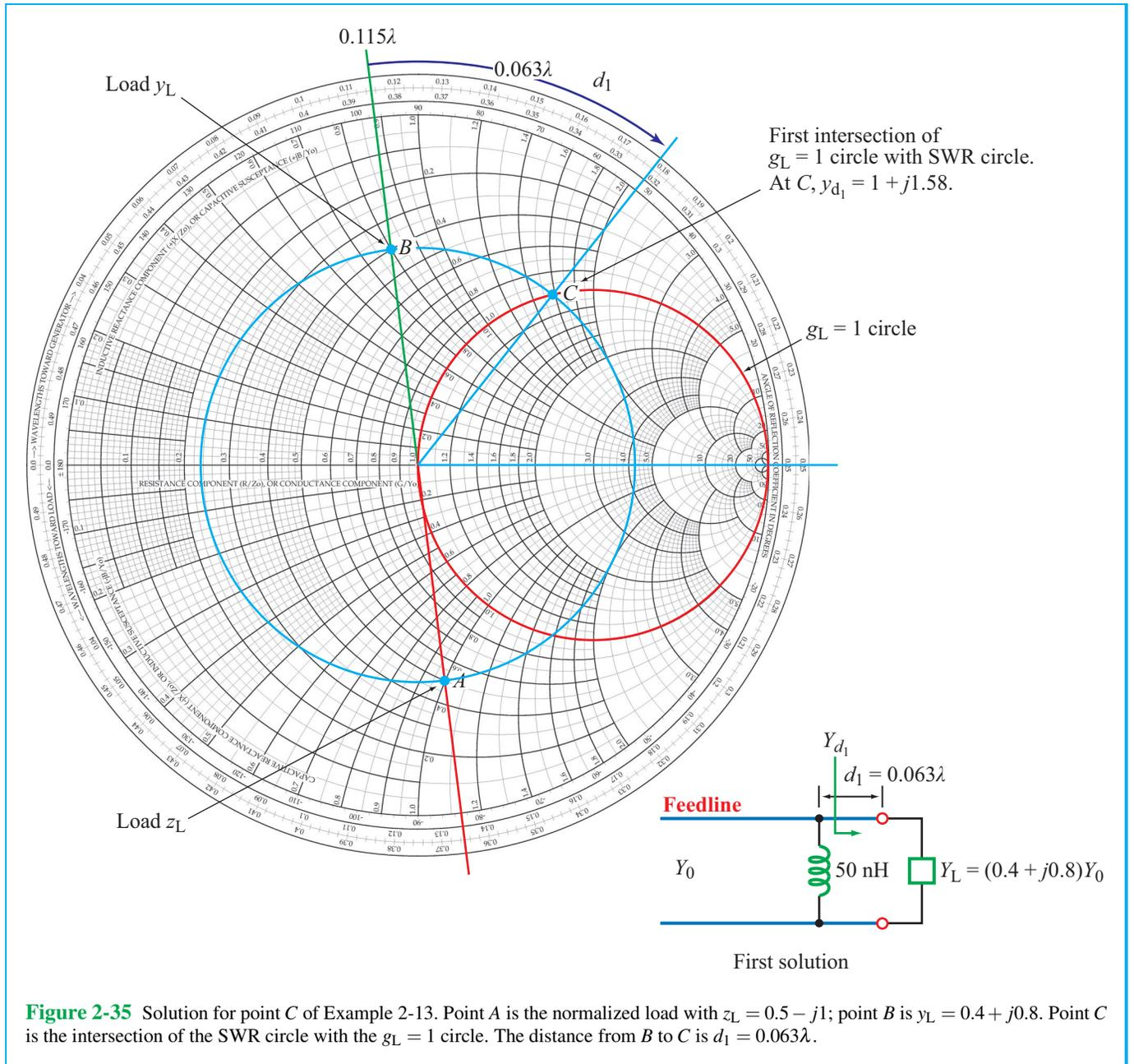
**Figure 2-35** Solution for point C of Example 2-13. Point A is the normalized load with  $z_L = 0.5 - j1$ ; point B is  $y_L = 0.4 + j0.8$ . Point C is the intersection of the SWR circle with the  $g_L = 1$  circle. The distance from B to C is  $d_1 = 0.063\lambda$ .
