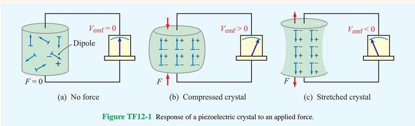
Figure TF12-1 Response of a piezoelectric crystal to an applied force.
