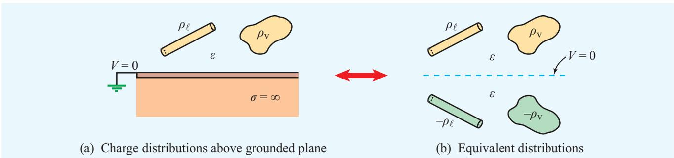
**Figure 4-31** Charge distributions above a conducting plane and their image-method equivalents.
