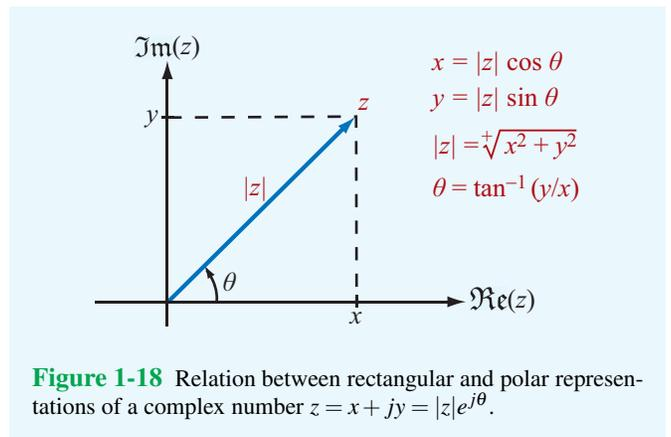
**Figure 1-18** Relation between rectangular and polar representations of a complex number  $z = x + jy = |z|e^{j\theta}$ .
