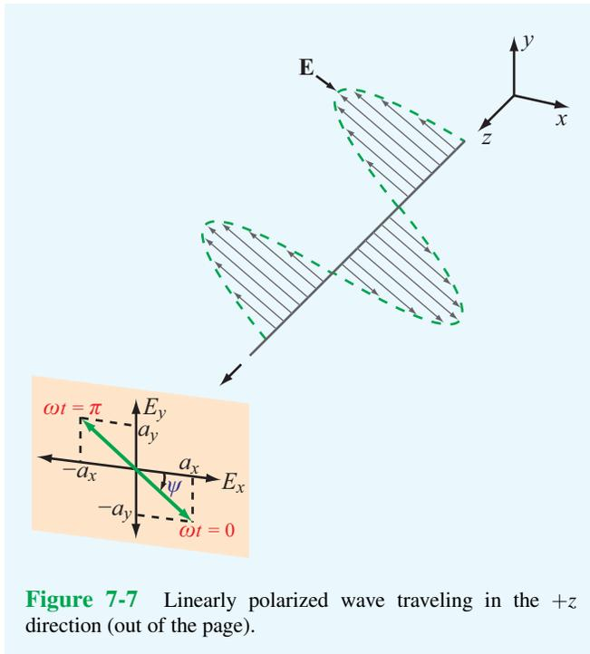
**Figure 7-7** Linearly polarized wave traveling in the +z direction (out of the page).
