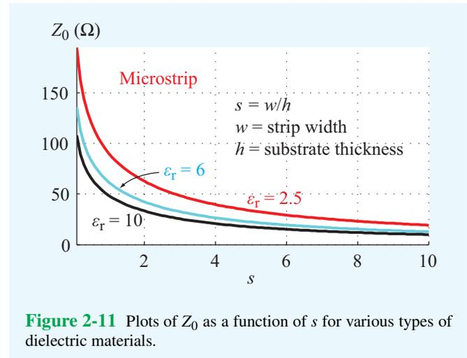
Figure 2-11 Plots of  $Z_0$  as a function of  $s$  for various types of dielectric materials.
