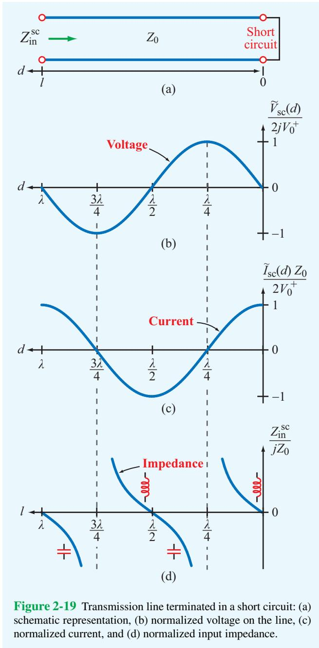
**Figure 2-19** Transmission line terminated in a short circuit: (a) schematic representation, (b) normalized voltage on the line, (c) normalized current, and (d) normalized input impedance.
