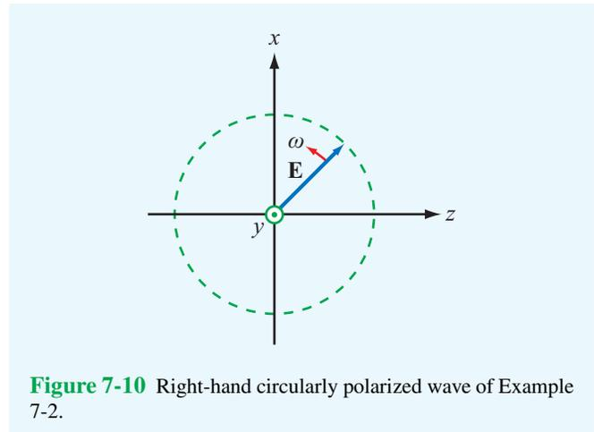
**Figure 7-10** Right-hand circularly polarized wave of Example 7-2.
