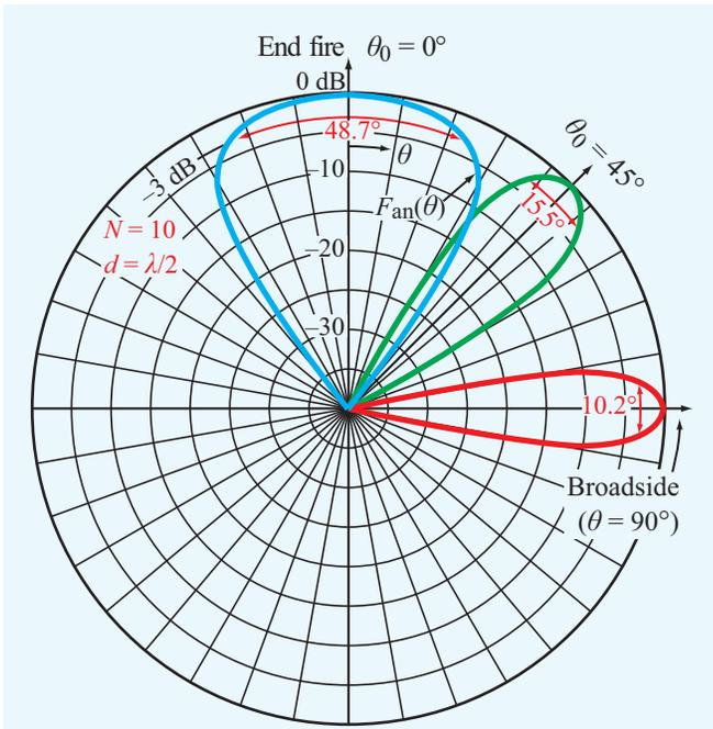
**Figure 9-33** Normalized array pattern of a 10-element array with  $\lambda/2$  spacing between adjacent elements. All elements are excited with equal amplitude. Through the application of linear phase across the array, the main beam can be steered from the broadside direction ( $\theta_0 = 90^\circ$ ) to any scan angle  $\theta_0$ . Equiphas excitation corresponds to  $\theta_0 = 90^\circ$ .
