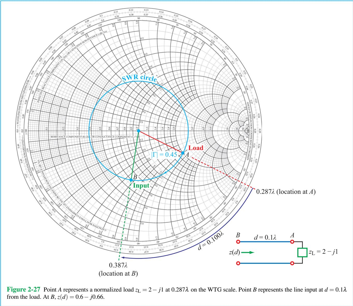
**Figure 2-27** Point A represents a normalized load  $z_L = 2 - j1$  at  $0.287\lambda$  on the WTG scale. Point B represents the line input at  $d = 0.1\lambda$  from the load. At B,  $z(d) = 0.6 - j0.66$ .
