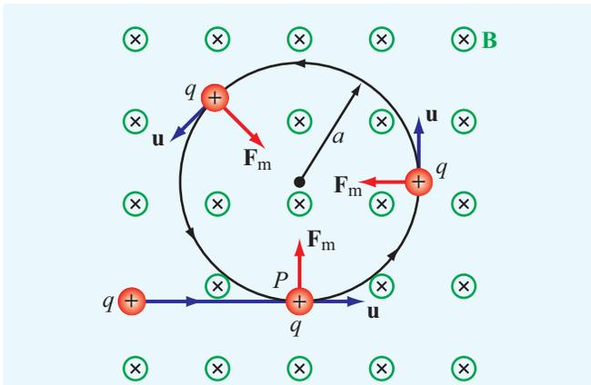
**Figure P5.3** Particle of charge  $q$  projected with velocity  $\mathbf{u}$  into a medium with a uniform field  $\mathbf{B}$  perpendicular to  $\mathbf{u}$  (Problem 5.3).
