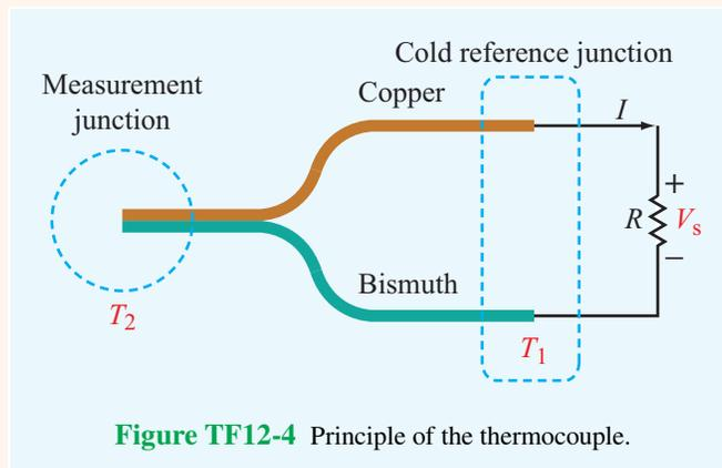
**Figure TF12-4** Principle of the thermocouple.
