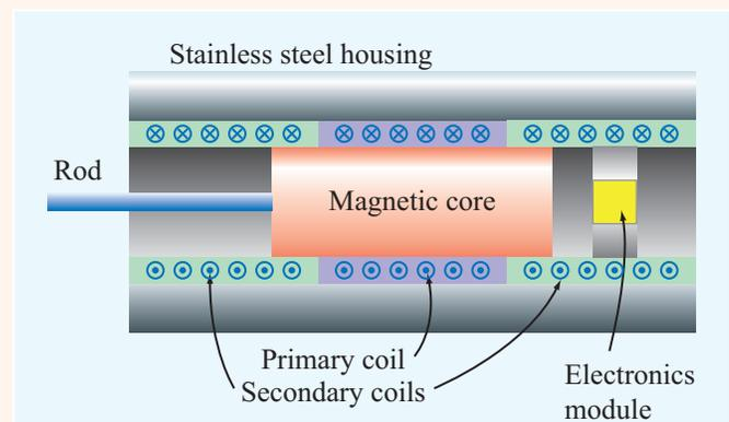
**Figure TF11-3** Cutaway view of LVDT.
