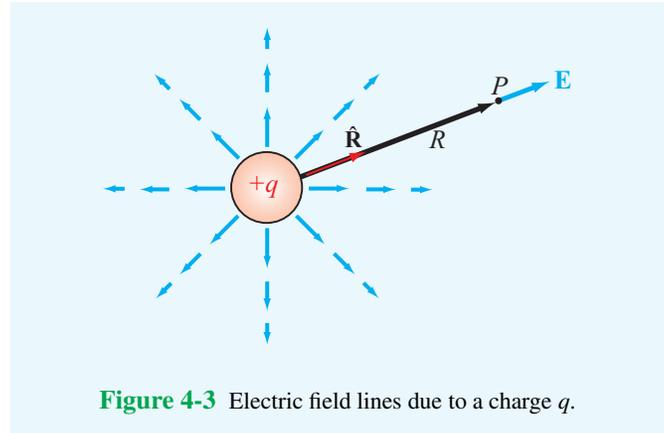
**Figure 4-3** Electric field lines due to a charge  $q$ .
