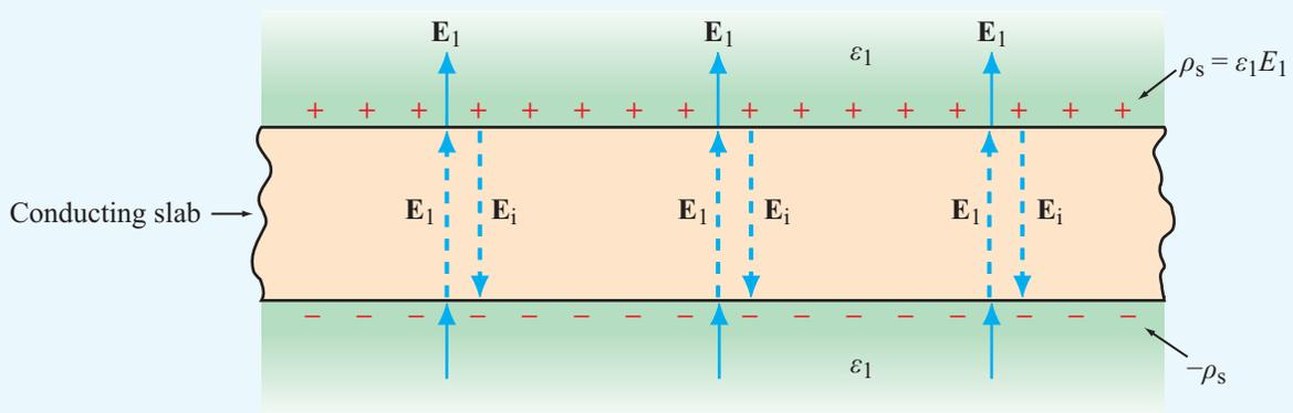
**Figure 4-22** When a conducting slab is placed in an external electric field  $\mathbf{E}_1$ , charges that accumulate on the conductor surfaces induce an internal electric field  $\mathbf{E}_i = -\mathbf{E}_1$ . Consequently, the total field inside the conductor is zero.
