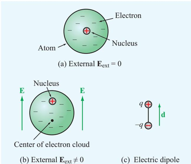
**Figure 4-18** In the absence of an external electric field  $\mathbf{E}$ , the center of the electron cloud is co-located with the center of the nucleus, but when a field is applied, the two centers are separated by a distance  $d$ .
