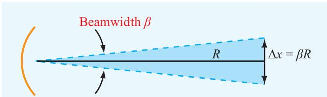
**Figure 10-12** The azimuth resolution  $\Delta x$  at a range  $R$  is equal to  $\beta R$ .
