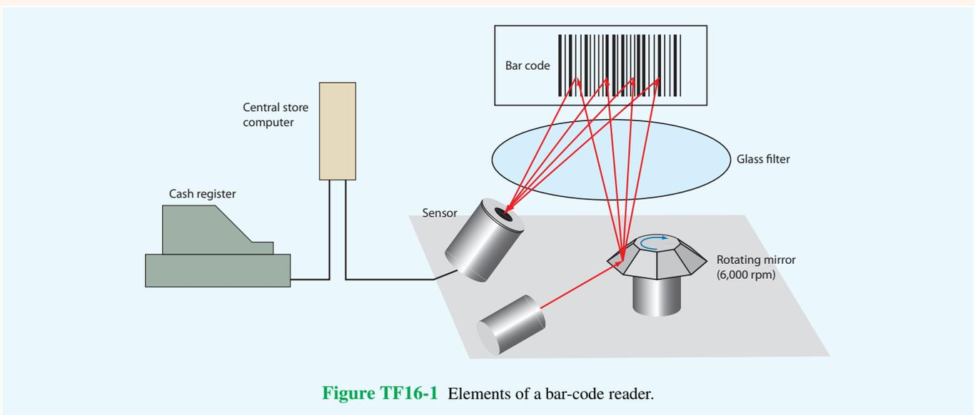
**Figure TF16-1** Elements of a bar-code reader.
