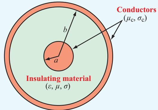
**Figure 2-7** Cross section of a coaxial line with inner conductor of radius  $a$  and outer conductor of radius  $b$ . The conductors have magnetic permeability  $\mu_c$  and conductivity  $\sigma_c$ , and the spacing material between the conductors has permittivity  $\epsilon$ , permeability  $\mu$ , and conductivity  $\sigma$ .
