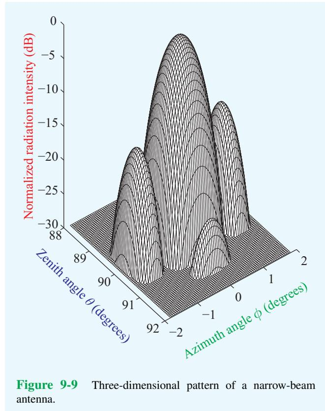
Figure 9-9 Three-dimensional pattern of a narrow-beam antenna.
