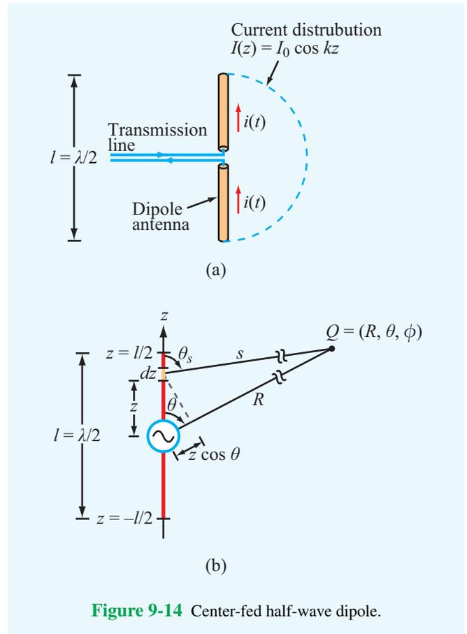
**Figure 9-14** Center-fed half-wave dipole.
