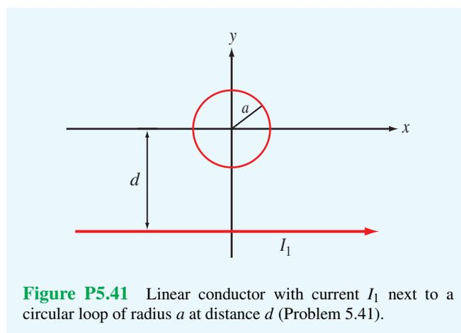
**Figure P5.41** Linear conductor with current  $I_1$  next to a circular loop of radius  $a$  at distance  $d$  (Problem 5.41).
