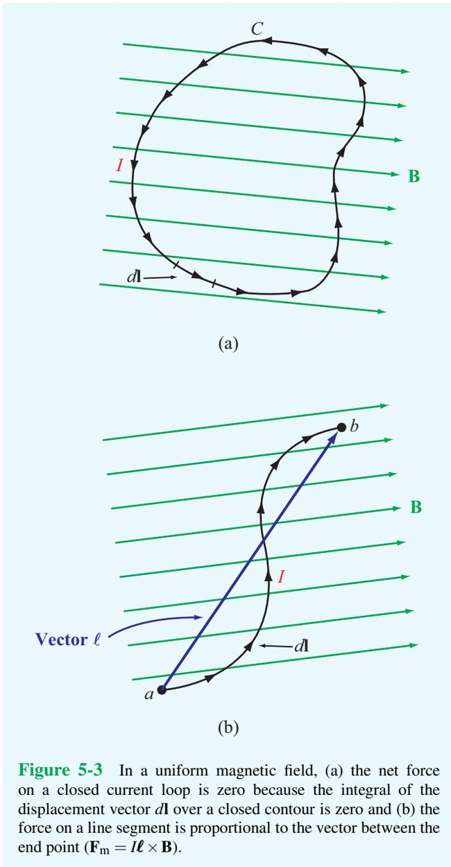
**Figure 5-3** In a uniform magnetic field, (a) the net force on a closed current loop is zero because the integral of the displacement vector  $d\mathbf{l}$  over a closed contour is zero and (b) the force on a line segment is proportional to the vector between the end point ( $\mathbf{F}_m = I\boldsymbol{\ell} \times \mathbf{B}$ ).
