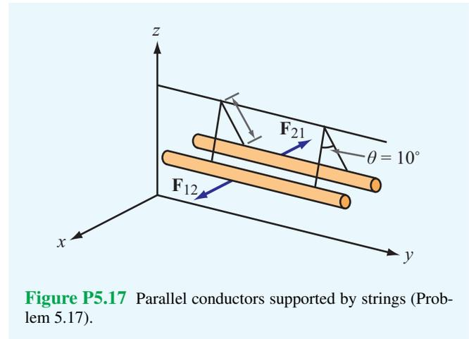
**Figure P5.17** Parallel conductors supported by strings (Problem 5.17).
