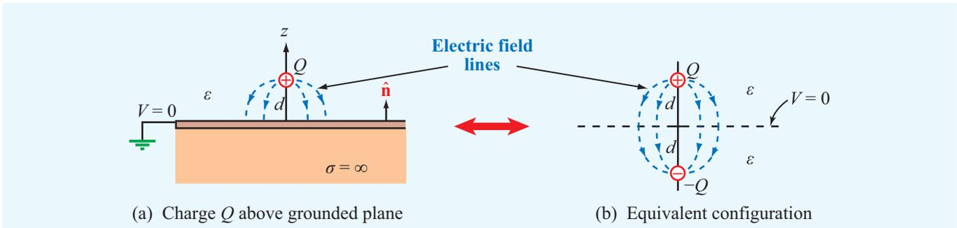
**Figure 4-30** By image theory, a charge  $Q$  above a grounded, perfectly conducting plane is equivalent to  $Q$  and its image  $-Q$  with the grounded plane removed.
