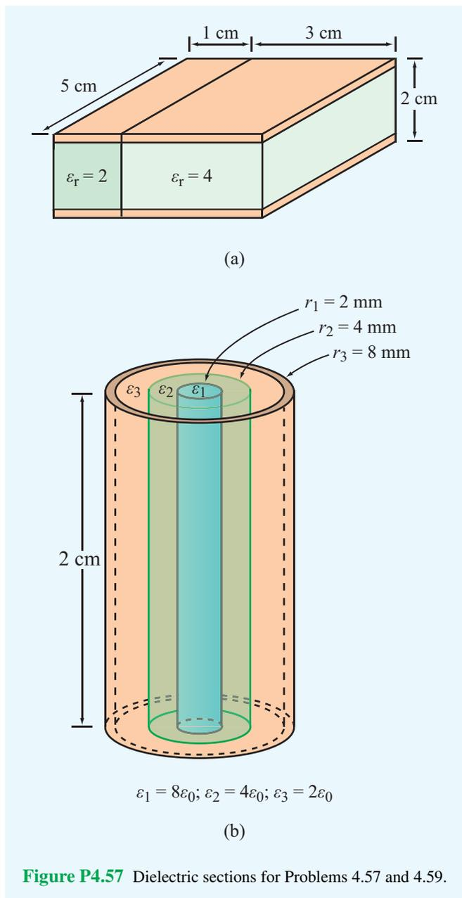
**Figure P4.57** Dielectric sections for Problems 4.57 and 4.59.
