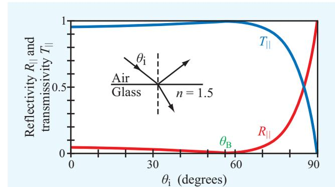
**Figure 8-19** Angular plots for  $(R_{\parallel}, T_{\parallel})$  for an air–glass interface.
