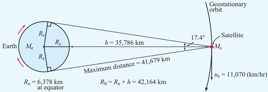
**Figure 10-3** Satellite of mass  $m_s$  in orbit around Earth. For the orbit to be geostationary, the distance  $R_0$  between the satellite and Earth's center should be 42,164 km. At the equator, this corresponds to an altitude of 35,786 km above Earth's surface.
