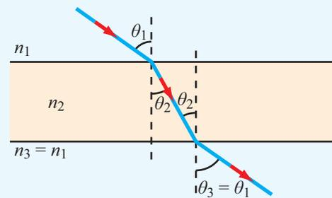
**Figure 8-11** The exit angle  $\theta_3$  is equal to the incidence angle  $\theta_1$  if the dielectric slab has parallel boundaries and is surrounded by media with the same index of refraction on both sides (Example 8-4).
