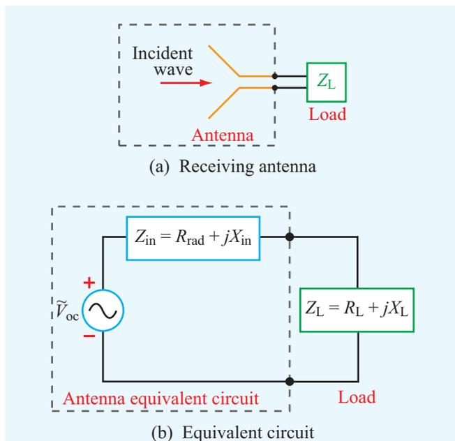
**Figure 9-18** Receiving antenna represented by an equivalent circuit.
