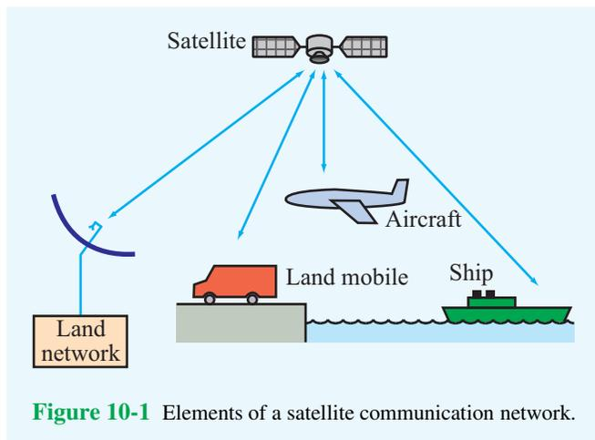
Figure 10-1 Elements of a satellite communication network.
