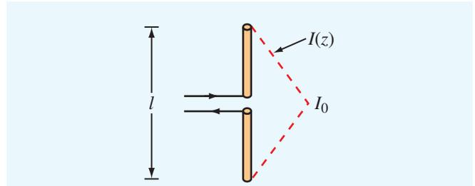
**Figure P9.15** Triangular current distribution on a short dipole (Problem 9.15).
