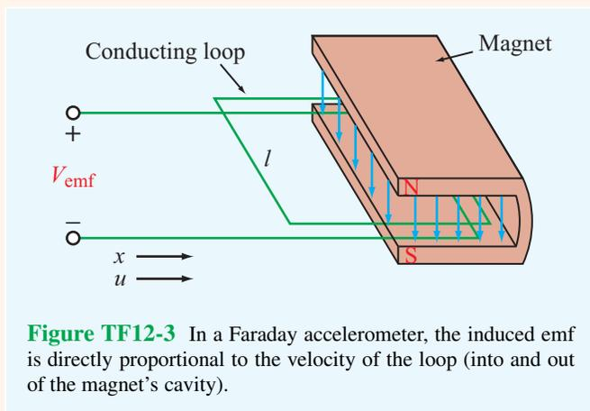
**Figure TF12-3** In a Faraday accelerometer, the induced emf is directly proportional to the velocity of the loop (into and out of the magnet's cavity).
