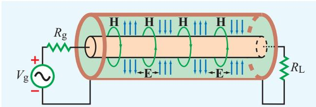
**Figure 7-3** A guided electromagnetic wave traveling in a coaxial transmission line consists of time-varying electric and magnetic fields in the dielectric medium between the inner and outer conductors.
