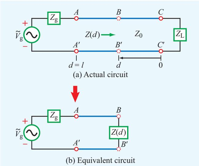
**Figure 2-17** The segment to the right of terminals  $BB'$  can be replaced with a discrete impedance equal to the wave impedance  $Z(d)$ .
