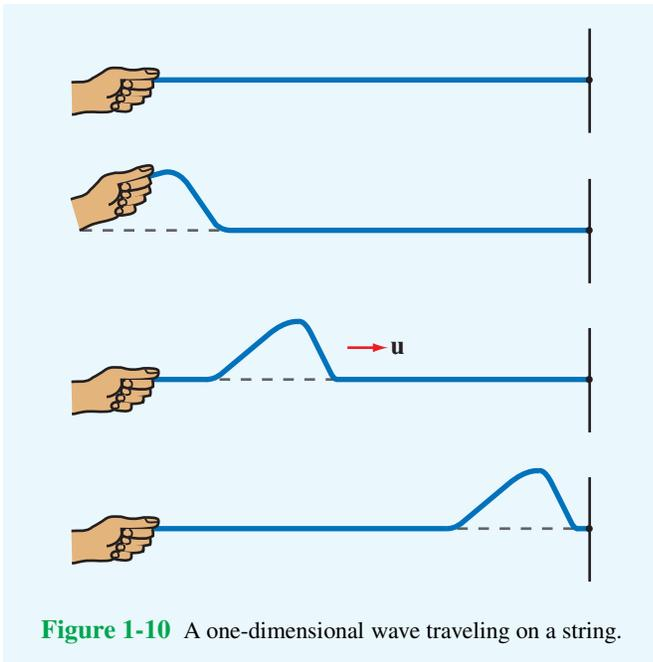
**Figure 1-10** A one-dimensional wave traveling on a string.
