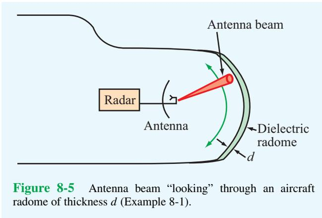
**Figure 8-5** Antenna beam “looking” through an aircraft radome of thickness  $d$  (Example 8-1).
