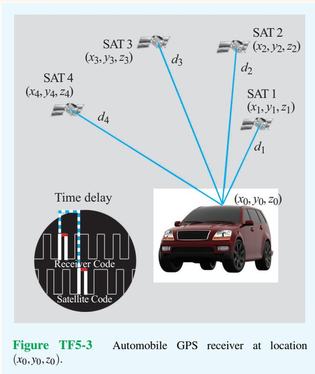
**Figure TF5-3** Automobile GPS receiver at location  $(x_0, y_0, z_0)$ .
