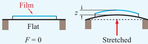
Figure TF7-3 Piezoresistor films.
