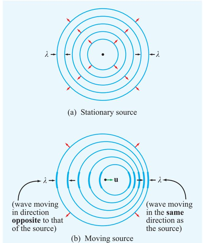
**Figure 10-15** A wave radiated from a point source when (a) stationary and (b) moving. The wave is compressed in the direction of motion, spread out in the opposite direction, and unaffected in the direction normal to motion.
