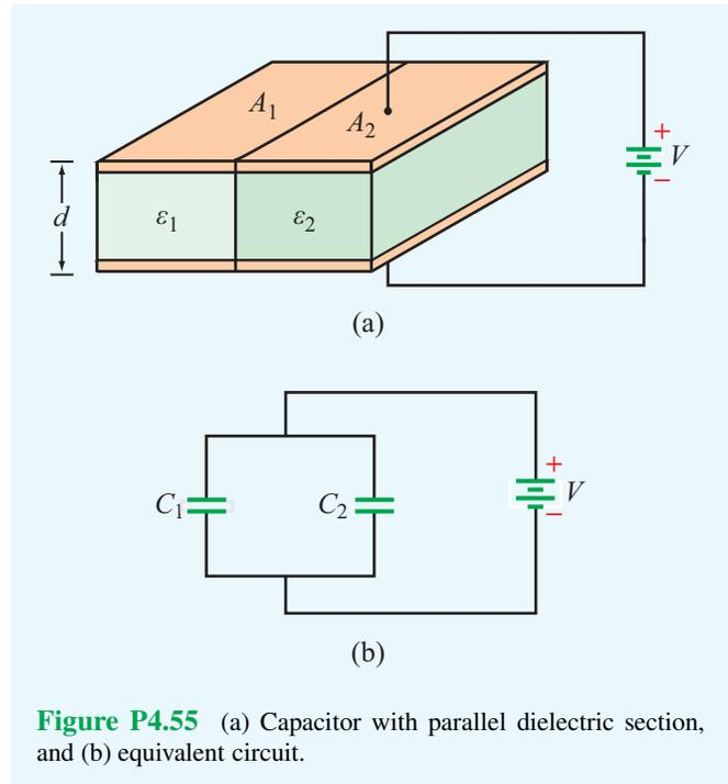
**Figure P4.55** (a) Capacitor with parallel dielectric section, and (b) equivalent circuit.
