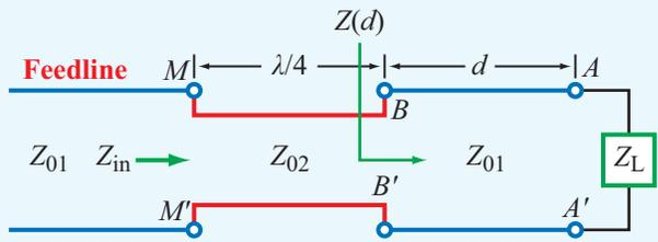
(b) If  $Z_L = \text{complex}$ : in-series  $\lambda/4$  transformer inserted at  $d = d_{\text{max}}$  or  $d = d_{\text{min}}$
