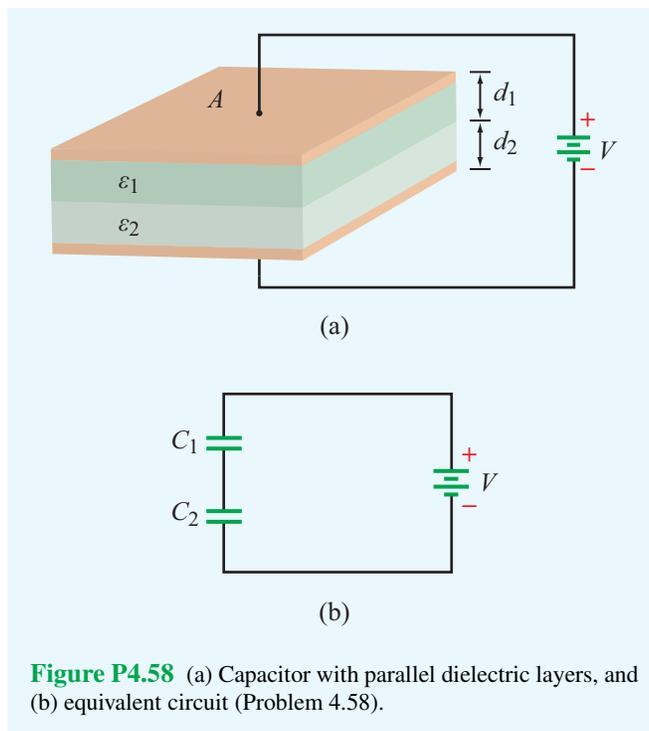
**Figure P4.58** (a) Capacitor with parallel dielectric layers, and (b) equivalent circuit (Problem 4.58).
