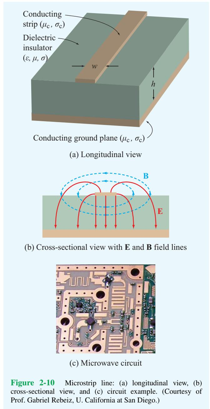
**Figure 2-10** Microstrip line: (a) longitudinal view, (b) cross-sectional view, and (c) circuit example. (Courtesy of Prof. Gabriel Rebeiz, U. California at San Diego.)
