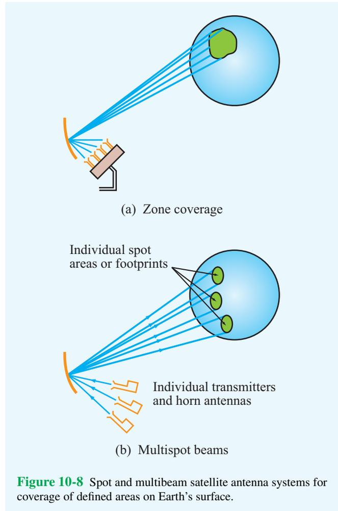
**Figure 10-8** Spot and multibeam satellite antenna systems for coverage of defined areas on Earth's surface.
