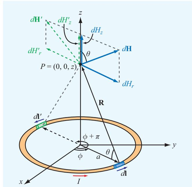
Figure 5-12 Circular loop carrying a current  $I$  (Example 5-3).
