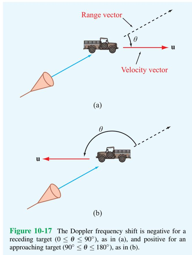
**Figure 10-17** The Doppler frequency shift is negative for a receding target ( $0 \leq \theta \leq 90^\circ$ ), as in (a), and positive for an approaching target ( $90^\circ \leq \theta \leq 180^\circ$ ), as in (b).
