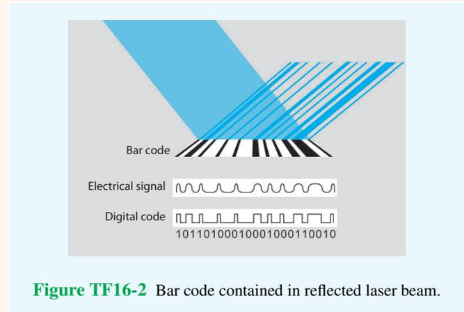
**Figure TF16-2** Bar code contained in reflected laser beam.
