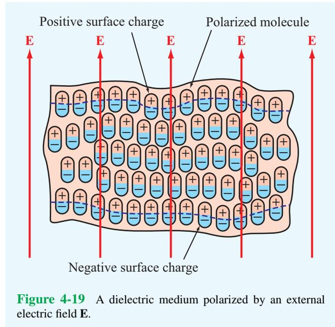
**Figure 4-19** A dielectric medium polarized by an external electric field  $\mathbf{E}$ .
