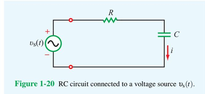
**Figure 1-20** RC circuit connected to a voltage source  $v_s(t)$ .
