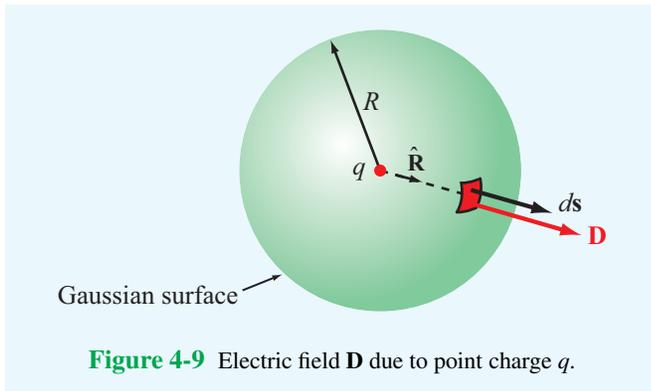
**Figure 4-9** Electric field  $\mathbf{D}$  due to point charge  $q$ .
