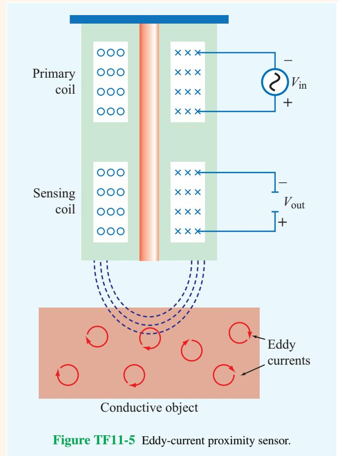
**Figure TF11-5** Eddy-current proximity sensor.
