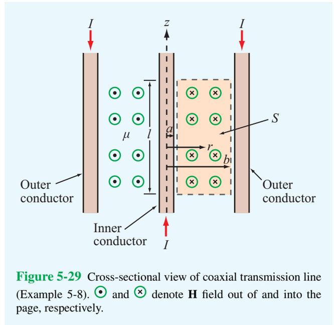
**Figure 5-29** Cross-sectional view of coaxial transmission line (Example 5-8).  $\odot$  and  $\otimes$  denote  $\mathbf{H}$  field out of and into the page, respectively.
