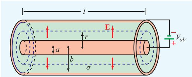
Figure 4-17 Coaxial cable of Example 4-11.
