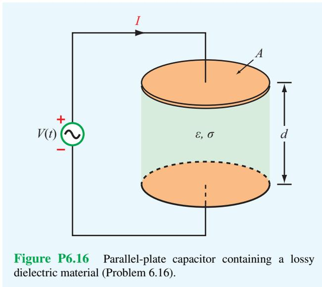
Figure P6.16 Parallel-plate capacitor containing a lossy dielectric material (Problem 6.16).
