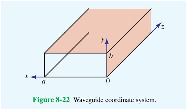
Figure 8-22 Waveguide coordinate system.
