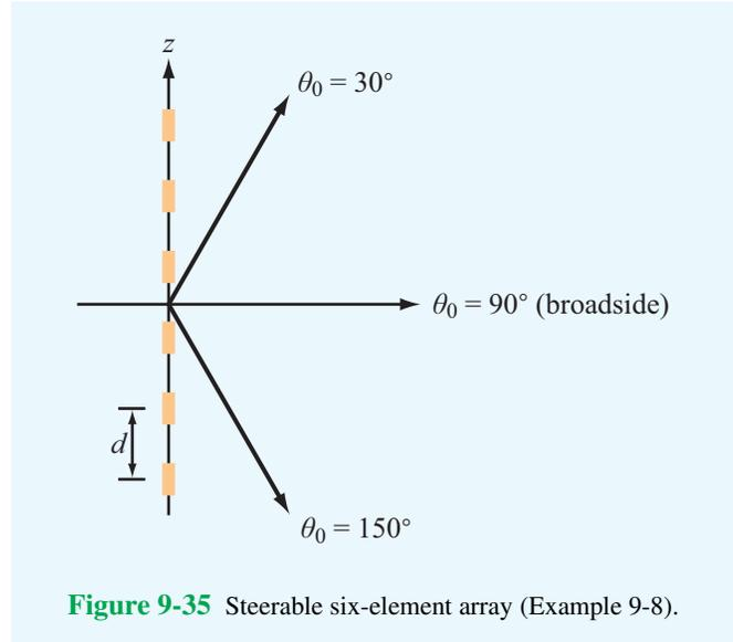
Figure 9-35 Steerable six-element array (Example 9-8).
