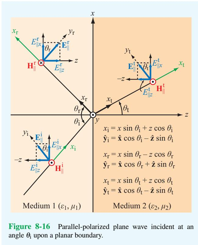
**Figure 8-16** Parallel-polarized plane wave incident at an angle  $\theta_i$  upon a planar boundary.
