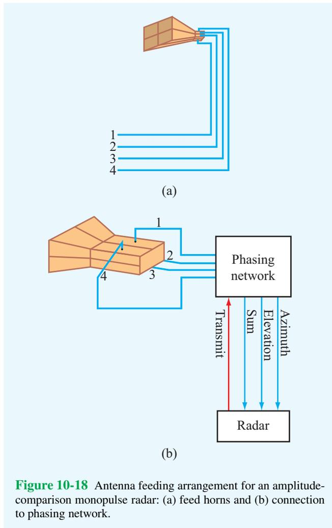
**Figure 10-18** Antenna feeding arrangement for an amplitude-comparison monopulse radar: (a) feed horns and (b) connection to phasing network.
