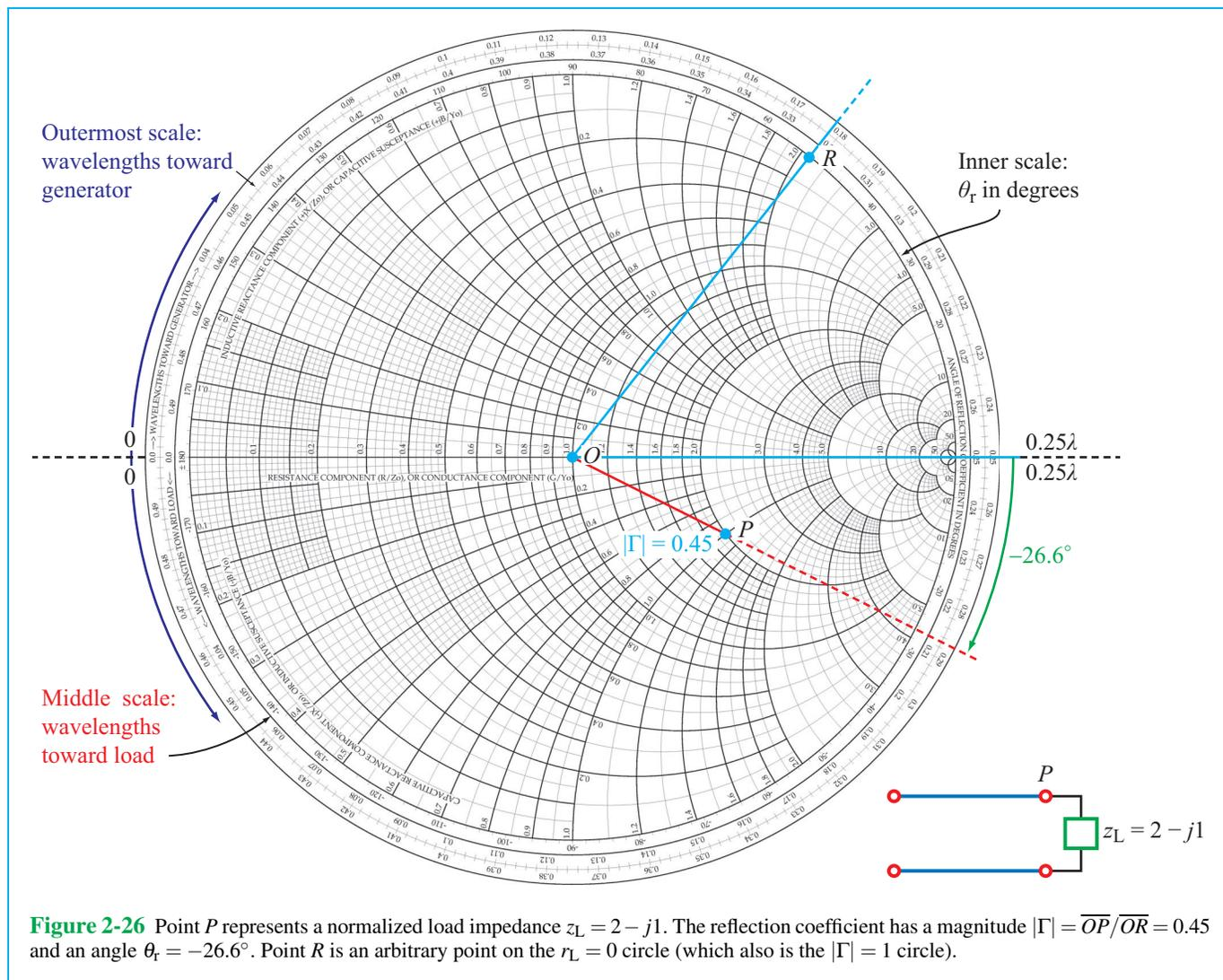
**Figure 2-26** Point  $P$  represents a normalized load impedance  $z_L = 2 - j1$ . The reflection coefficient has a magnitude  $|\Gamma| = \overline{OP}/\overline{OR} = 0.45$  and an angle  $\theta_r = -26.6^\circ$ . Point  $R$  is an arbitrary point on the  $r_L = 0$  circle (which also is the  $|\Gamma| = 1$  circle).
