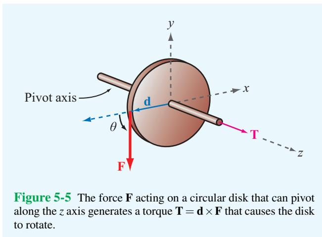
**Figure 5-5** The force  $\mathbf{F}$  acting on a circular disk that can pivot along the  $z$  axis generates a torque  $\mathbf{T} = \mathbf{d} \times \mathbf{F}$  that causes the disk to rotate.
