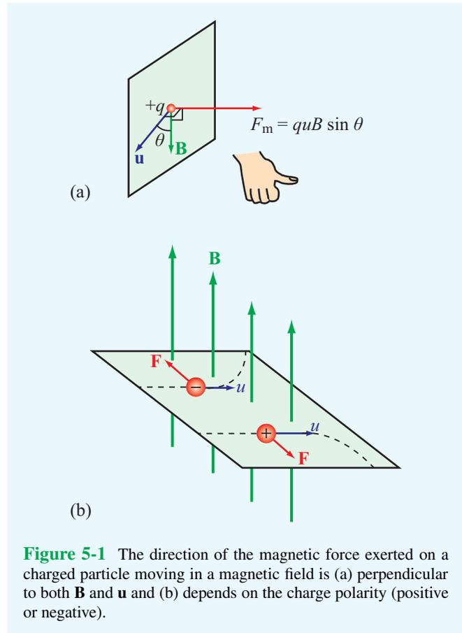
**Figure 5-1** The direction of the magnetic force exerted on a charged particle moving in a magnetic field is (a) perpendicular to both  $\mathbf{B}$  and  $\mathbf{u}$  and (b) depends on the charge polarity (positive or negative).
