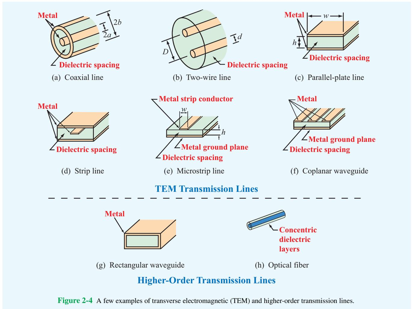
**Figure 2-4** A few examples of transverse electromagnetic (TEM) and higher-order transmission lines.
