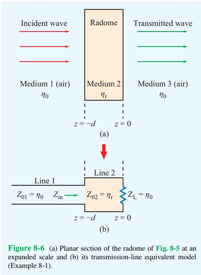
**Figure 8-6** (a) Planar section of the radome of Fig. 8-5 at an expanded scale and (b) its transmission-line equivalent model (Example 8-1).
