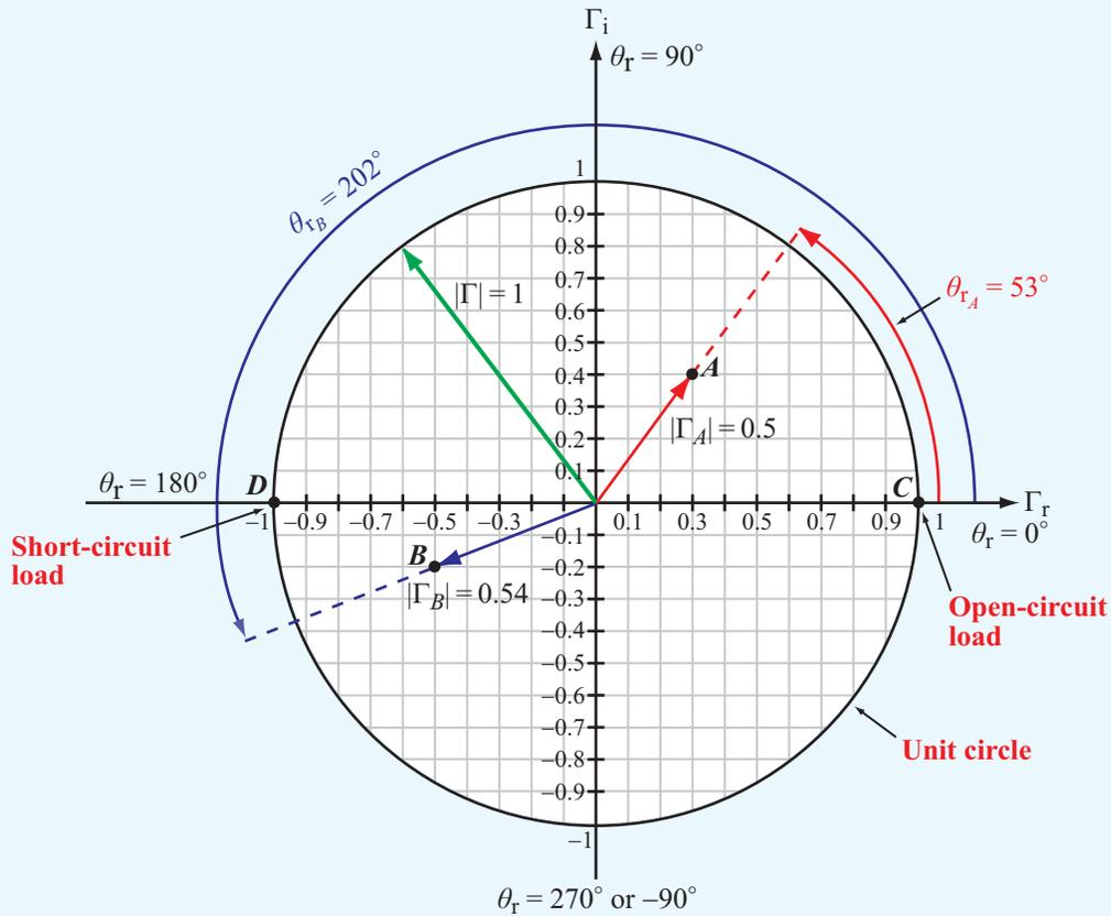
**Figure 2-24** The complex  $\Gamma$  plane. Point A is at  $\Gamma_A = 0.3 + j0.4 = 0.5e^{j53^\circ}$ , and point B is at  $\Gamma_B = -0.5 - j0.2 = 0.54e^{j202^\circ}$ . The unit circle corresponds to  $|\Gamma| = 1$ . At point C,  $\Gamma = 1$ , corresponding to an open-circuit load, and at point D,  $\Gamma = -1$ , corresponding to a short circuit.
