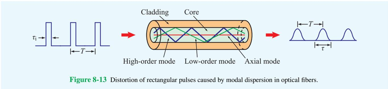
**Figure 8-13** Distortion of rectangular pulses caused by modal dispersion in optical fibers.
