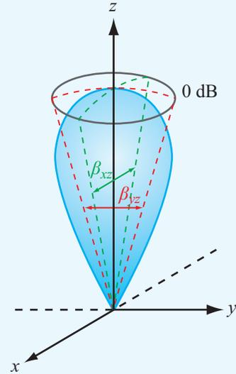
**Figure 9-12** The solid angle of a unidirectional radiation pattern is approximately equal to the product of the half-power beamwidths in the two principal planes; that is,  $\Omega_p \approx \beta_{xz}\beta_{yz}$ .
