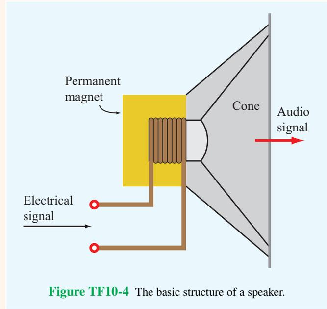
Figure TF10-4 The basic structure of a speaker.
