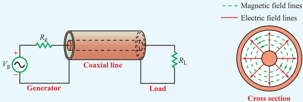
**Figure 2-5** In a coaxial line, the electric field is in the radial direction between the inner and outer conductors, and the magnetic field forms circles around the inner conductor. The coaxial line is a transverse electromagnetic (TEM) transmission line because both the electric and magnetic fields are orthogonal to the direction of propagation between the generator and the load.
