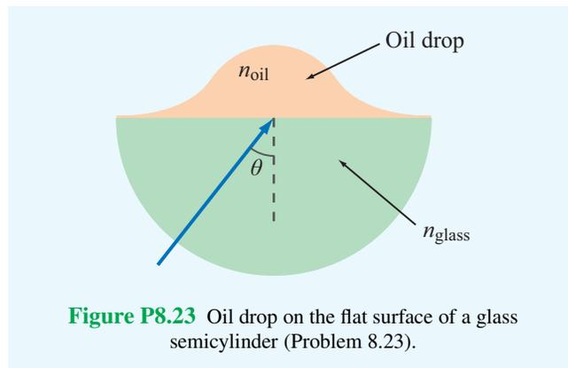
**Figure P8.23** Oil drop on the flat surface of a glass semicylinder (Problem 8.23).
