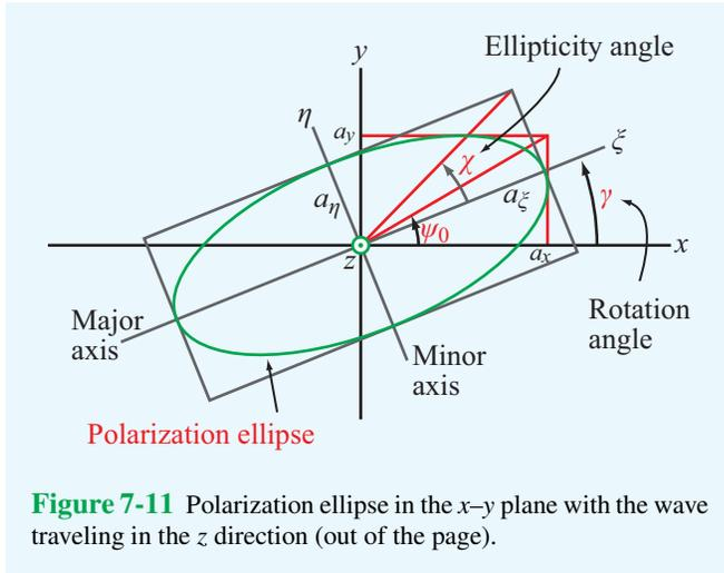
**Figure 7-11** Polarization ellipse in the  $x$ - $y$  plane with the wave traveling in the  $z$  direction (out of the page).
