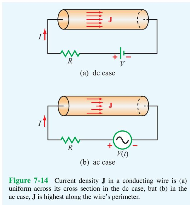
**Figure 7-14** Current density  $\mathbf{J}$  in a conducting wire is (a) uniform across its cross section in the dc case, but (b) in the ac case,  $\mathbf{J}$  is highest along the wire's perimeter.
