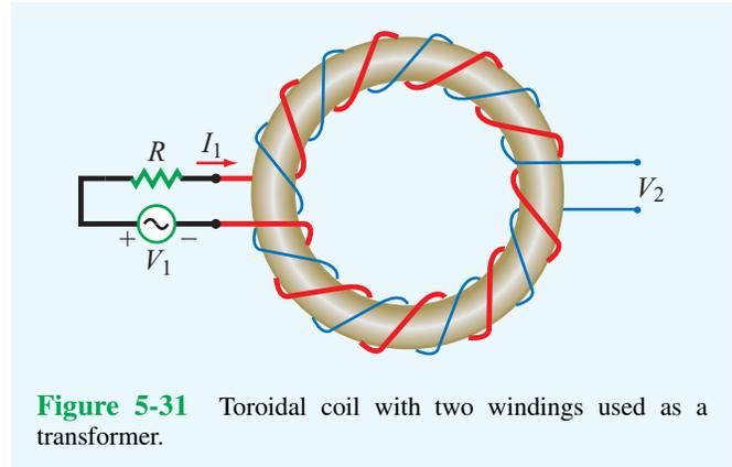
**Figure 5-31** Toroidal coil with two windings used as a transformer.
