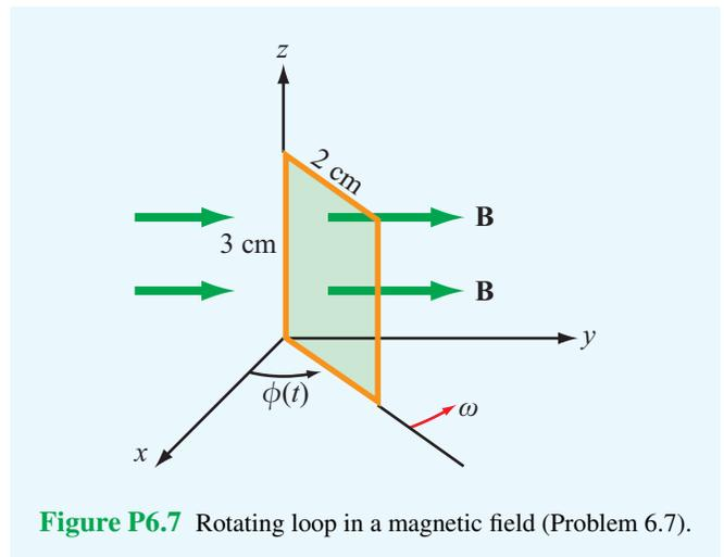
Figure P6.7 Rotating loop in a magnetic field (Problem 6.7).
