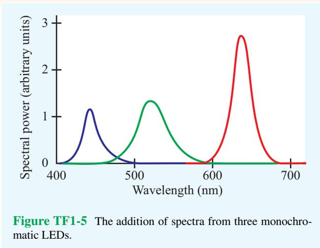
► The wavelength of the emitted photon depends on the diode's semiconductor material. The materials most commonly used are aluminum gallium arsenide (AlGaAs) to generate **red light**, indium gallium nitride (InGaN) to generate **blue light**, and aluminum gallium phosphide (AlGaP) to generate **green light**. In each case, the emitted energy is confined to a narrow spectral band. ◀
