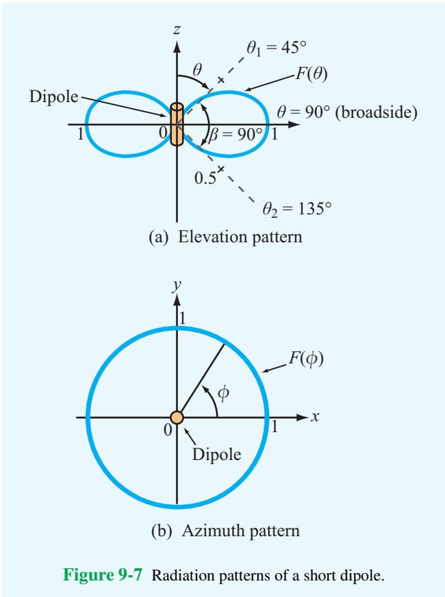
**Figure 9-7** Radiation patterns of a short dipole.
