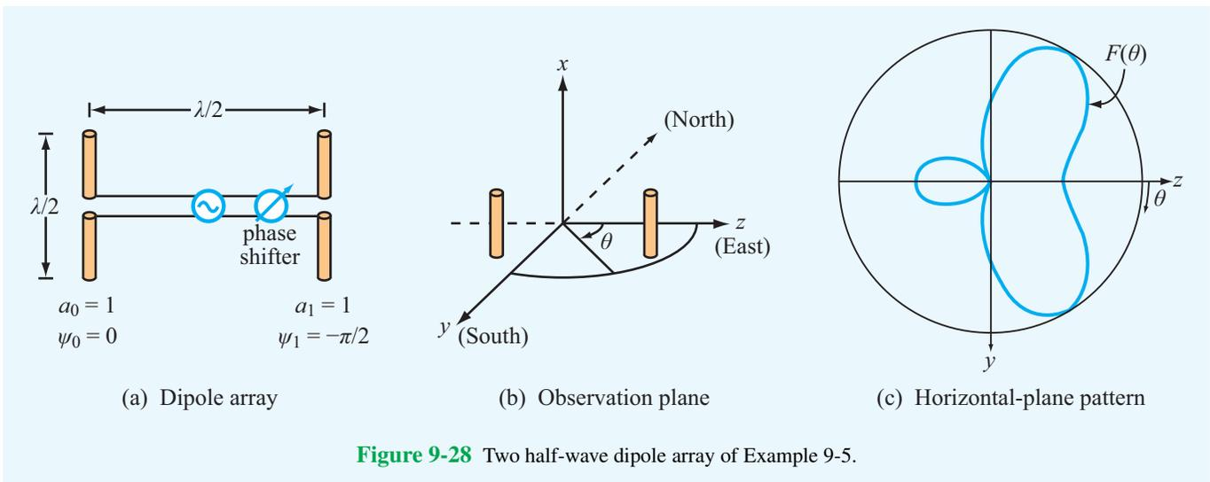
**Figure 9-28** Two half-wave dipole array of Example 9-5.
