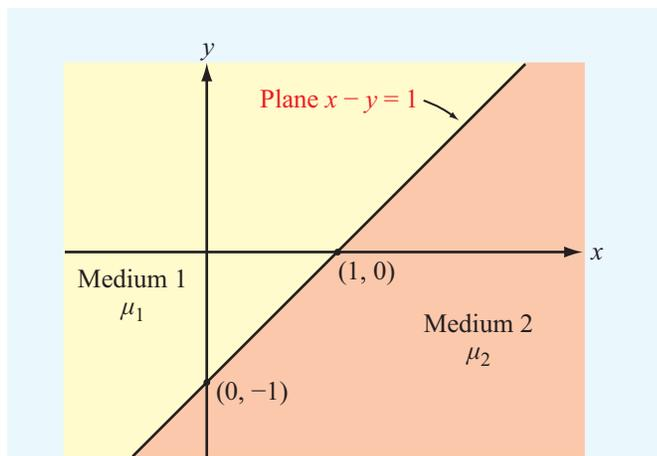
**Figure P5.34** Magnetic media separated by the plane  $x - y = 1$  (Problem 5.34).
