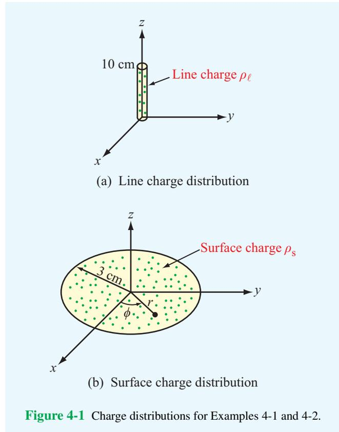
**Figure 4-1** Charge distributions for Examples 4-1 and 4-2.
