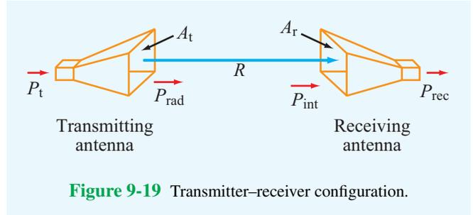
**Figure 9-19** Transmitter–receiver configuration.
