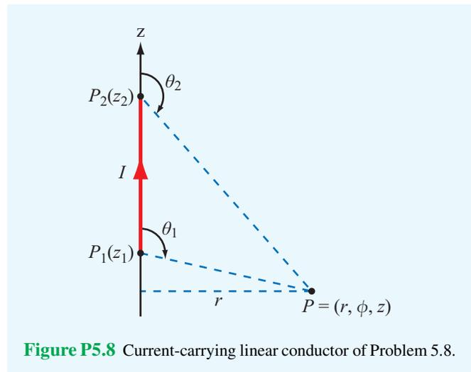
**Figure P5.8** Current-carrying linear conductor of Problem 5.8.
