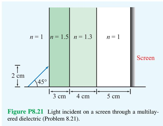
**Figure P8.21** Light incident on a screen through a multilayered dielectric (Problem 8.21).
