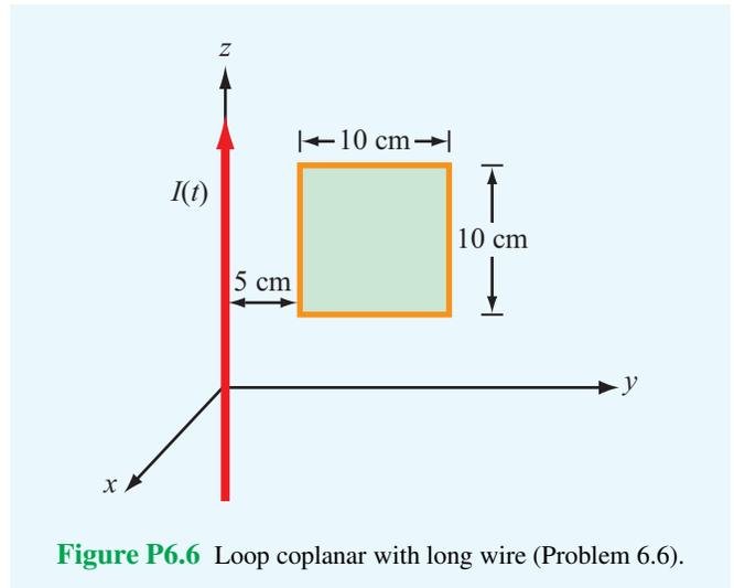
Figure P6.6 Loop coplanar with long wire (Problem 6.6).
