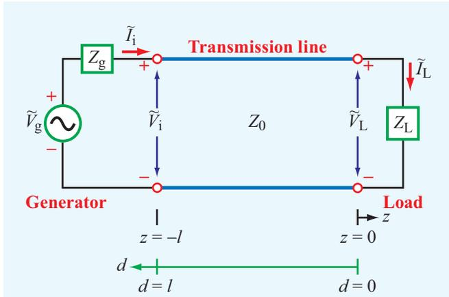
**Figure 2-12** Transmission line of length  $l$  connected on one end to a generator circuit and on the other end to a load  $Z_L$ . The load is located at  $z = 0$ , and the generator terminals are at  $z = -l$ . Coordinate  $d$  is defined as  $d = -z$ .
