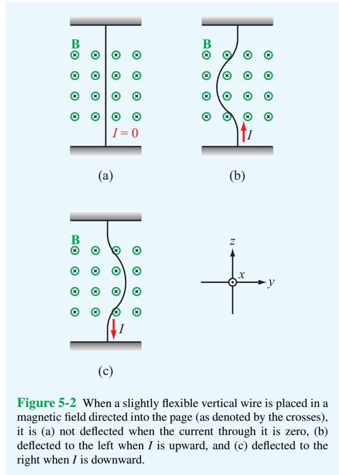
**Figure 5-2** When a slightly flexible vertical wire is placed in a magnetic field directed into the page (as denoted by the crosses), it is (a) not deflected when the current through it is zero, (b) deflected to the left when  $I$  is upward, and (c) deflected to the right when  $I$  is downward.
