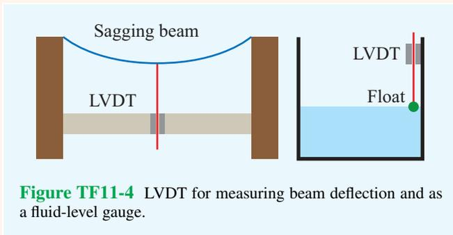
**Figure TF11-4** LVDT for measuring beam deflection and as a fluid-level gauge.
