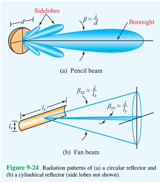
**Figure 9-24** Radiation patterns of (a) a circular reflector and (b) a cylindrical reflector (side lobes not shown).
