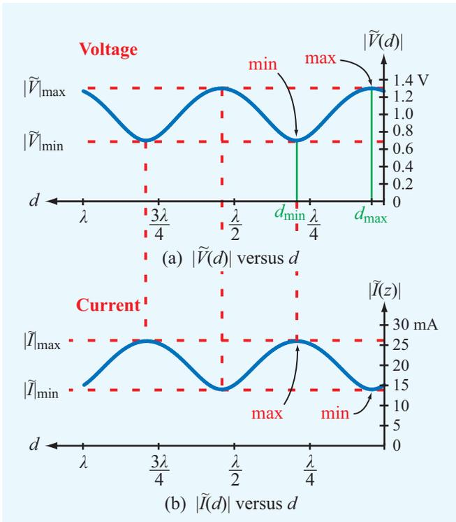
**Figure 2-14** Standing-wave pattern for (a)  $|\tilde{V}(d)|$  and (b)  $|\tilde{I}(d)|$  for a lossless transmission line of characteristic impedance  $Z_0 = 50 \Omega$ , terminated in a load with a reflection coefficient  $\Gamma = 0.3e^{j30^\circ}$ . The magnitude of the incident wave  $|V_0^+| = 1 \text{ V}$ . The standing-wave ratio is  $S = |\tilde{V}|_{\max}/|\tilde{V}|_{\min} = 1.3/0.7 = 1.86$ .
