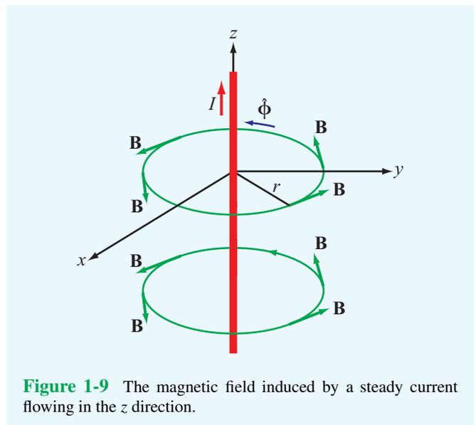
Figure 1-9 The magnetic field induced by a steady current flowing in the  $z$  direction.
