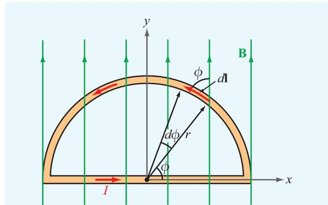
**Figure 5-4** Semicircular conductor in a uniform field (Example 5-1).
