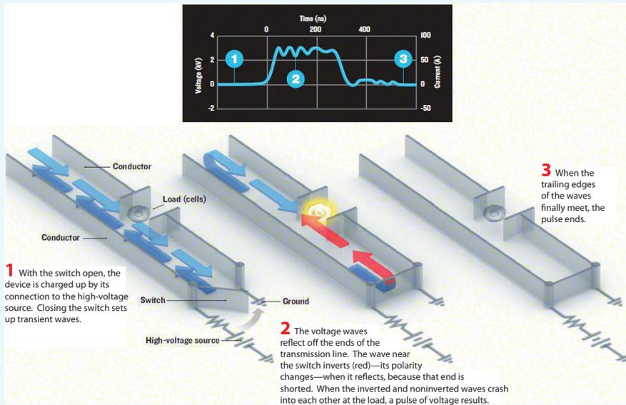
**Figure TF4-3** High-voltage nanosecond pulse delivered to tumor cells via a transmission line. The cells to be shocked by the pulse sit in a break in one of the transmission-line conductors. (Courtesy of *IEEE Spectrum*, August 2006.)
