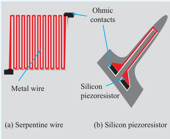
Figure TF7-4 Metal and silicon piezoresistors.
