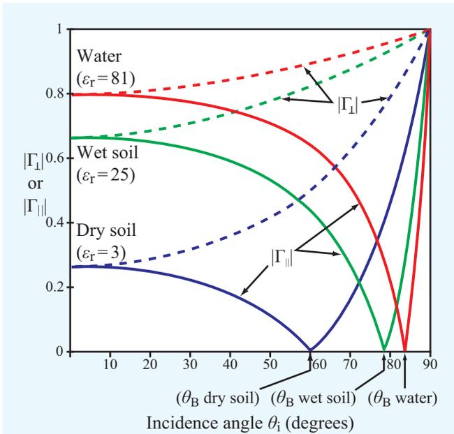
**Figure 8-17** Plots for  $|\Gamma_{\perp}|$  and  $|\Gamma_{\parallel}|$  as a function of  $\theta_i$  for a dry soil surface, a wet soil surface, and a water surface. For each surface,  $|\Gamma_{\parallel}| = 0$  at the Brewster angle.
