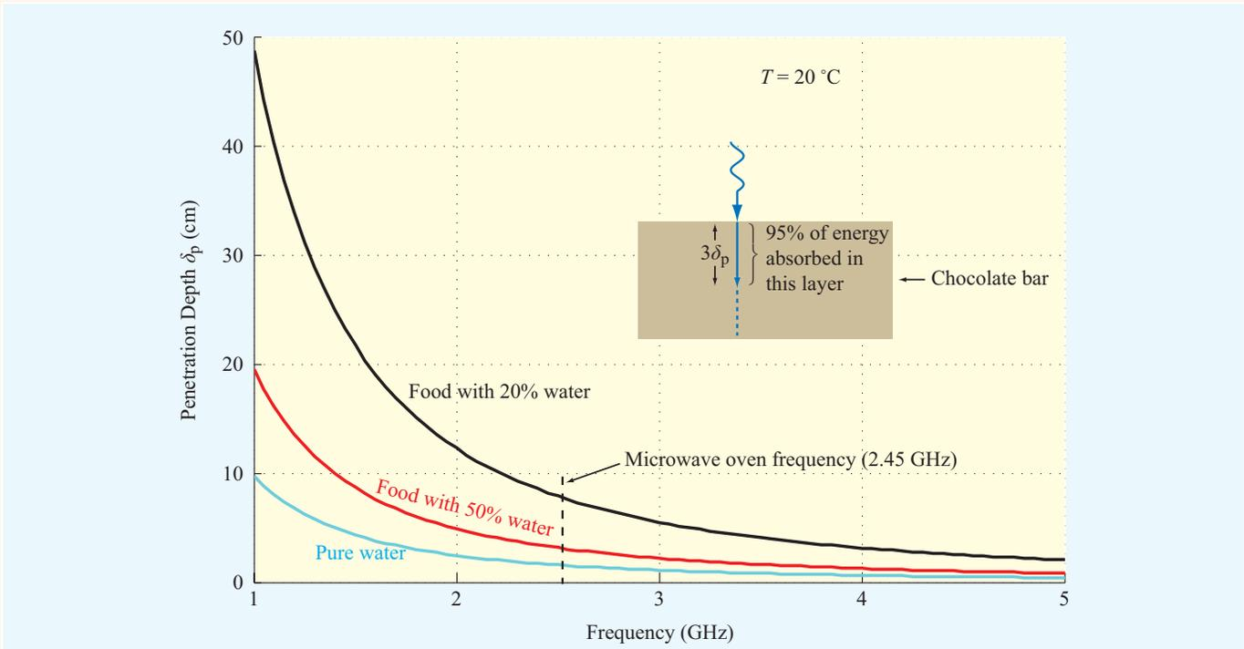
**Figure TF3-1** Penetration depth as a function of frequency (1–5 GHz) for pure water and two foods with different water contents.
