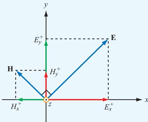
**Figure 7-6** The wave  $(\mathbf{E}, \mathbf{H})$  is equivalent to the sum of two waves: one with fields  $(E_x^+, H_y^+)$  and another with  $(E_y^+, H_x^+)$  with both traveling in the  $+z$  direction.
