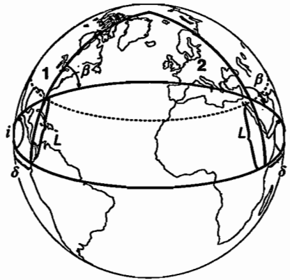
Fig. 6-12. Launch Window Geometry for Launches near the Ascending Node (1) and Descending Node (2). The angles shown are the orbital inclination ( i ), launch site latitude ( L ), and launch azimuth ( \beta ).
